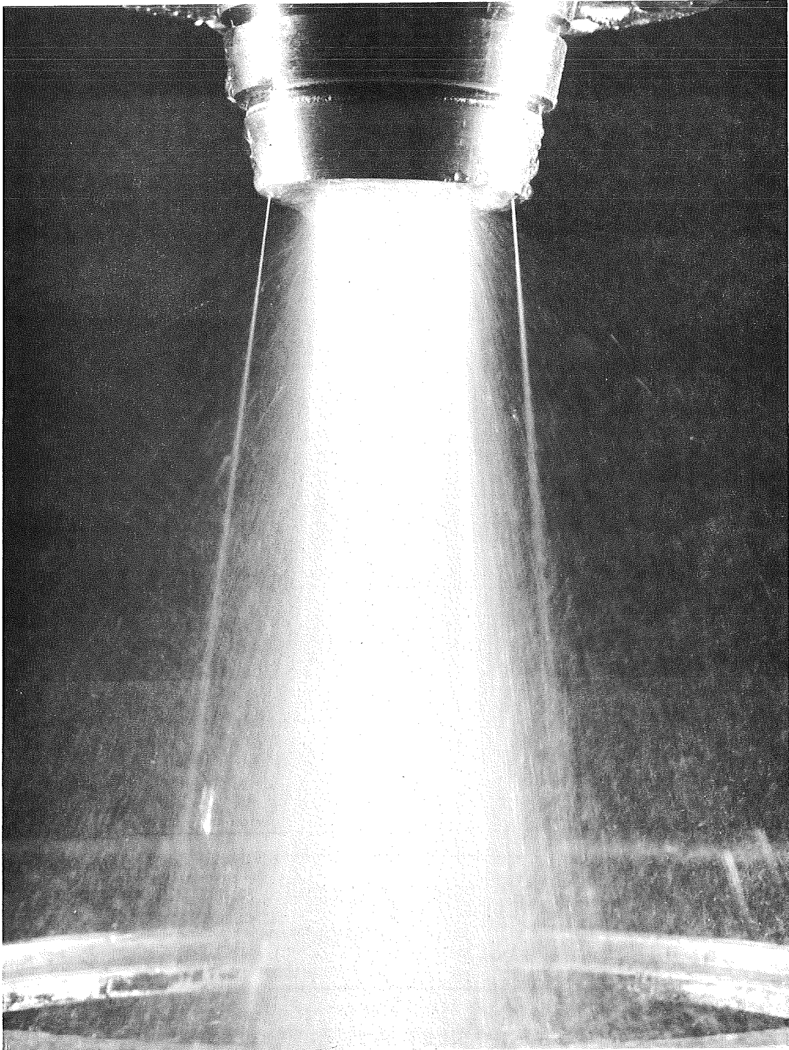
FIGURE 10. Total Spray Pattern from Water Flow Tests of the Serial No. 001 FLOX/Methane Injector
