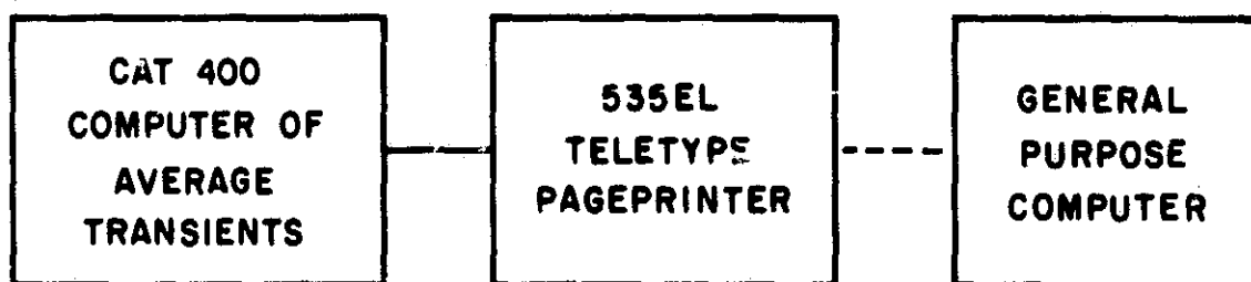
Figure 99. Coupling of CAT to the Computer for Batch Processing
