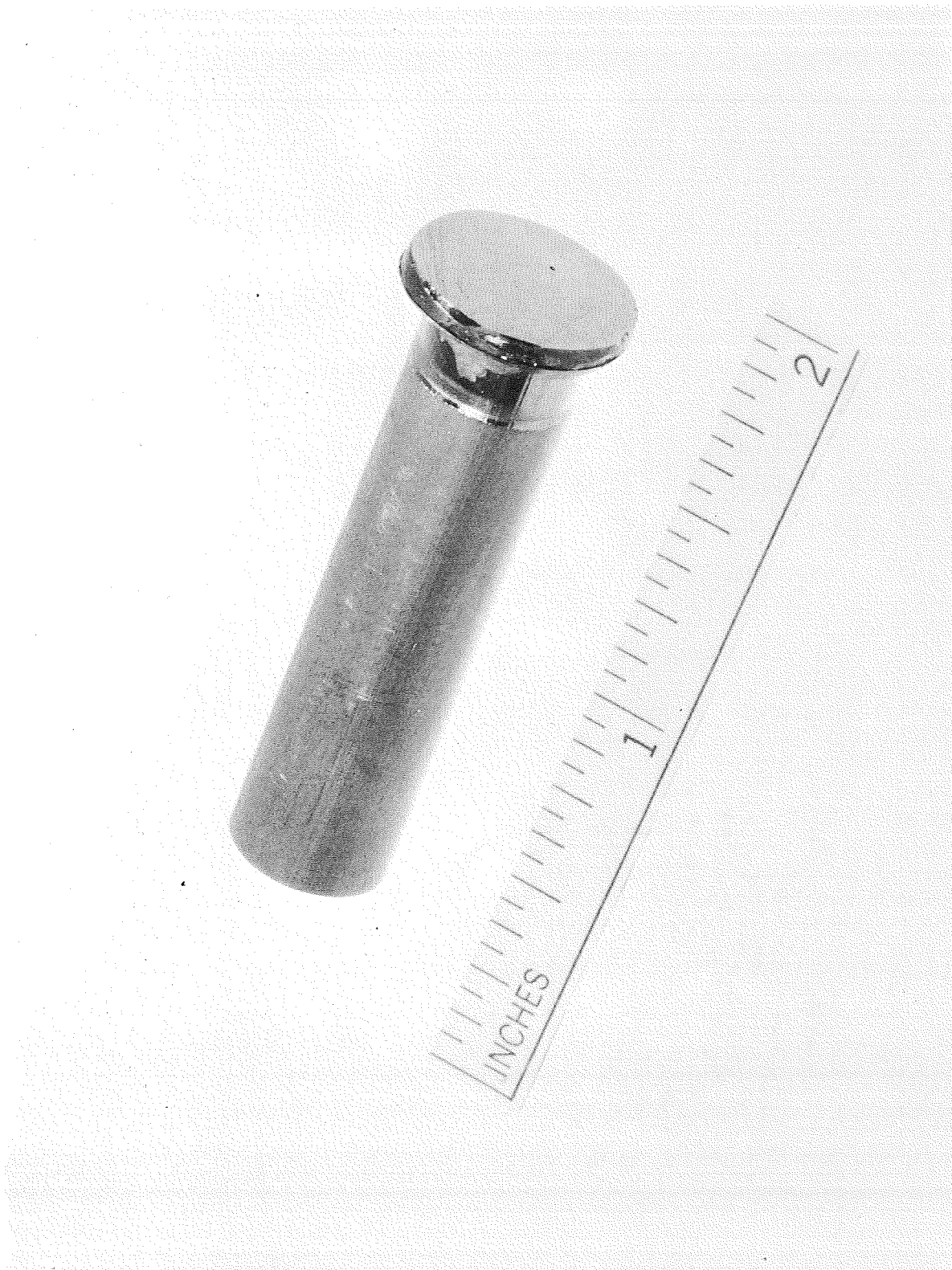
Figure 4-10. Gallium Arsenide Window Sealed to Molybdenum Tubing by Metal Soldering.
