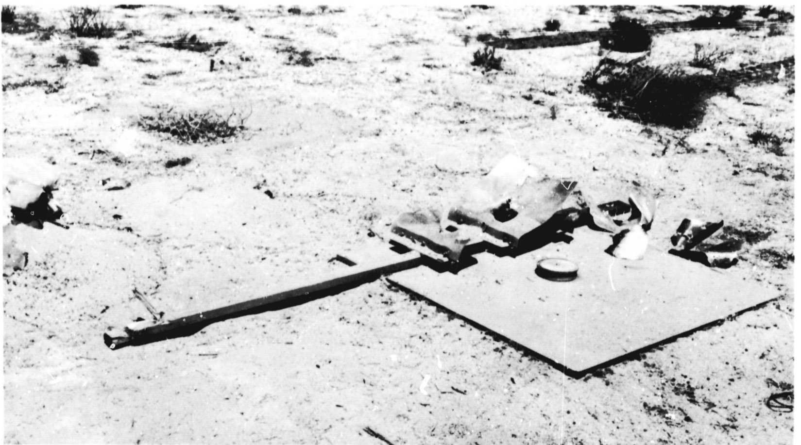
Fig. 6. Condition of plates after shaped-charge detonation
