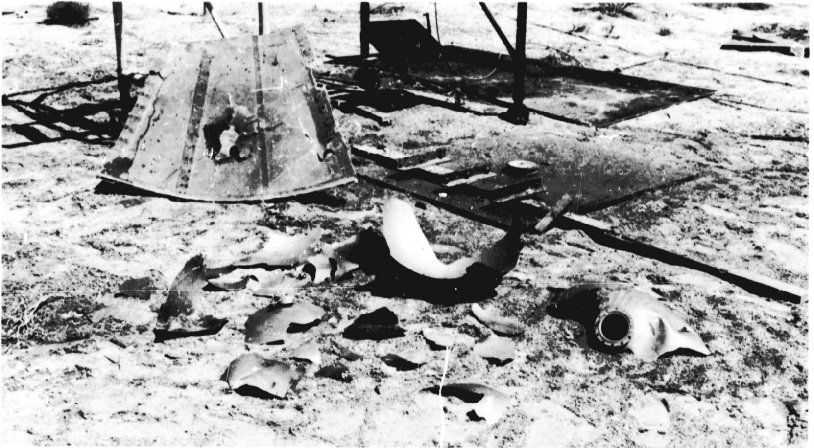
Fig. 9. Postfiring condition of tank and bulkhead
