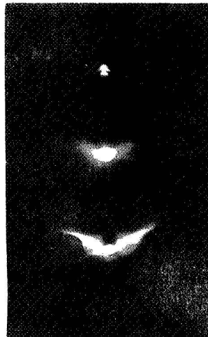
IMAGE CONVERTER CAMERA PHOTOGRAPH OF VACUUM BREAKDOWN (Aluminum Rods)
