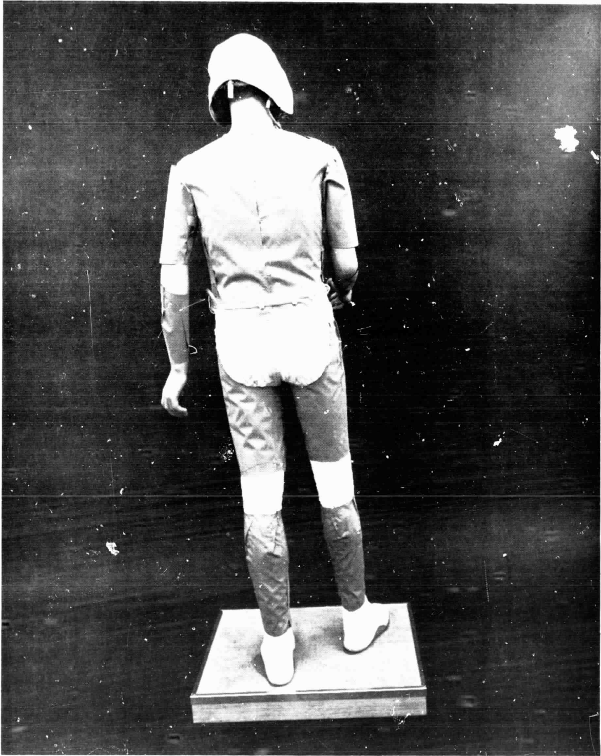
Figure 12. EECGS Patterns over Apollo LCG - Back View
