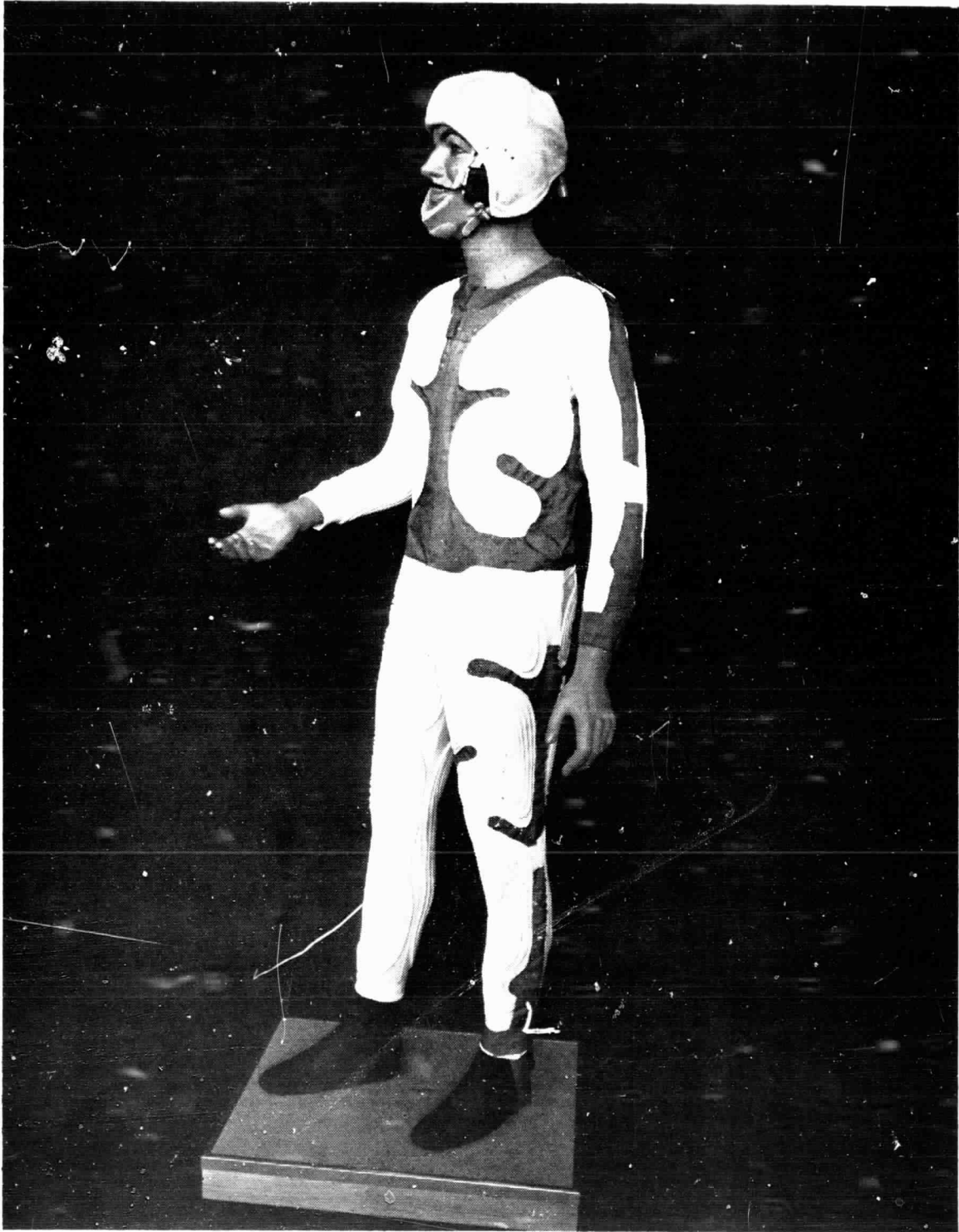
Figure 9. Unused Body Contact Areas British Frankenstein Beaufort LCG Type 1 Series 5 - Side View
