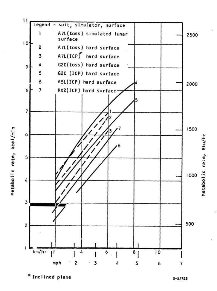
Figure 15. Comparison of A7L, G2C, A5L, and RX2 Pressure Suits
