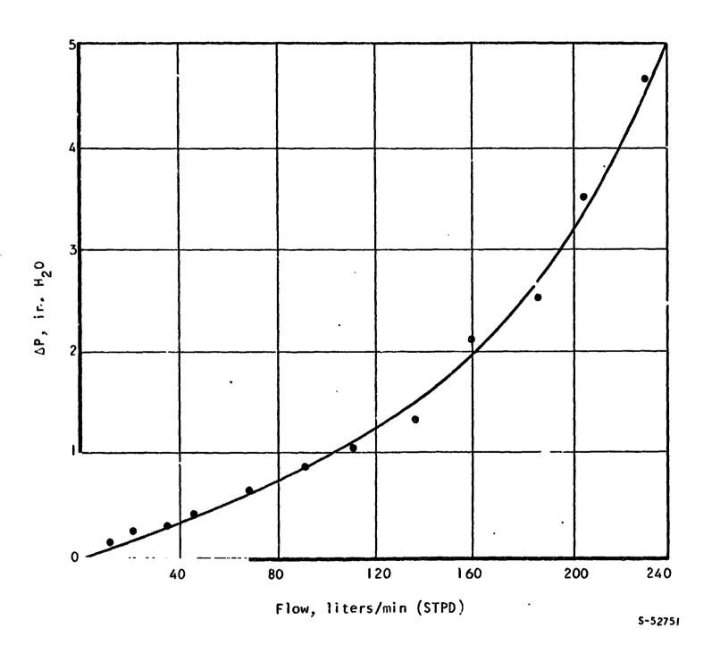
Figure II. Pressure Drop as a Function of Gas Flow Through the AiResearch Respiratory Valve System
