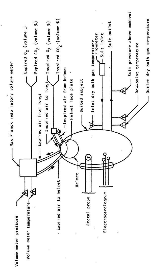
Figure 10. Schematic of the Basic Respiratory System
