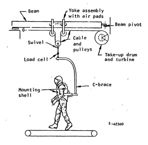
Figure 6. Turbine-Operated Suspension System
