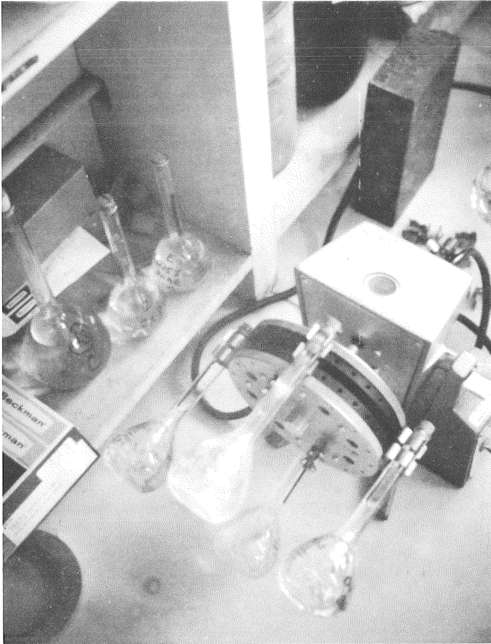
Fig. 4. Rotator modified by attached vertical volumetric flasks, each filled with agar or other suspending media to test medium-rotation interactions.
