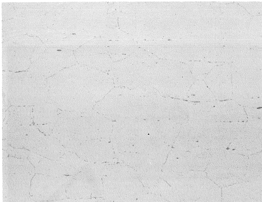
Fig. IV-8 Microstructure of Unaged, Cryogenically-Stretched Type 301 Stainless Steel; Parent Metal; Longitudinal Direction (Enlarged 250X)
