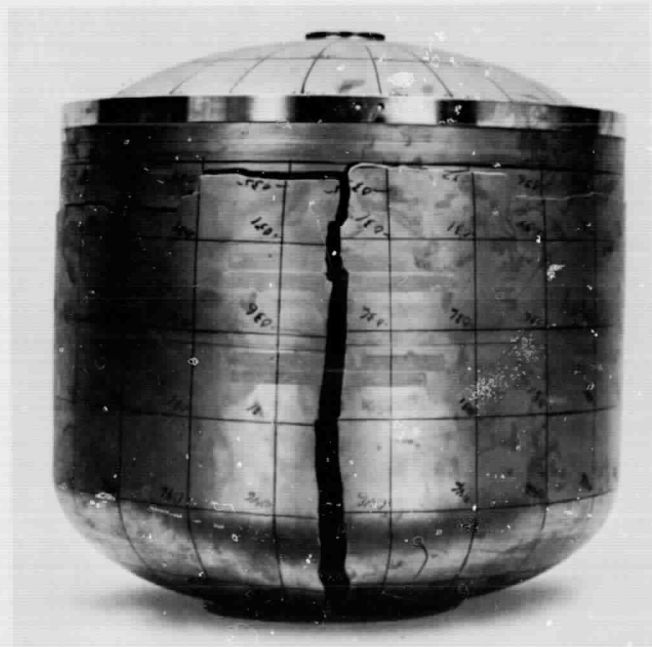
Fig. 9. Chamber B-1T after hydrostatic burst test
