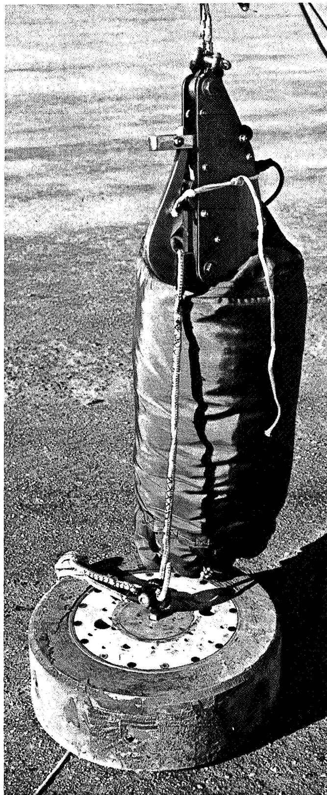
Fig. 4. Parachute pack for gliding test
