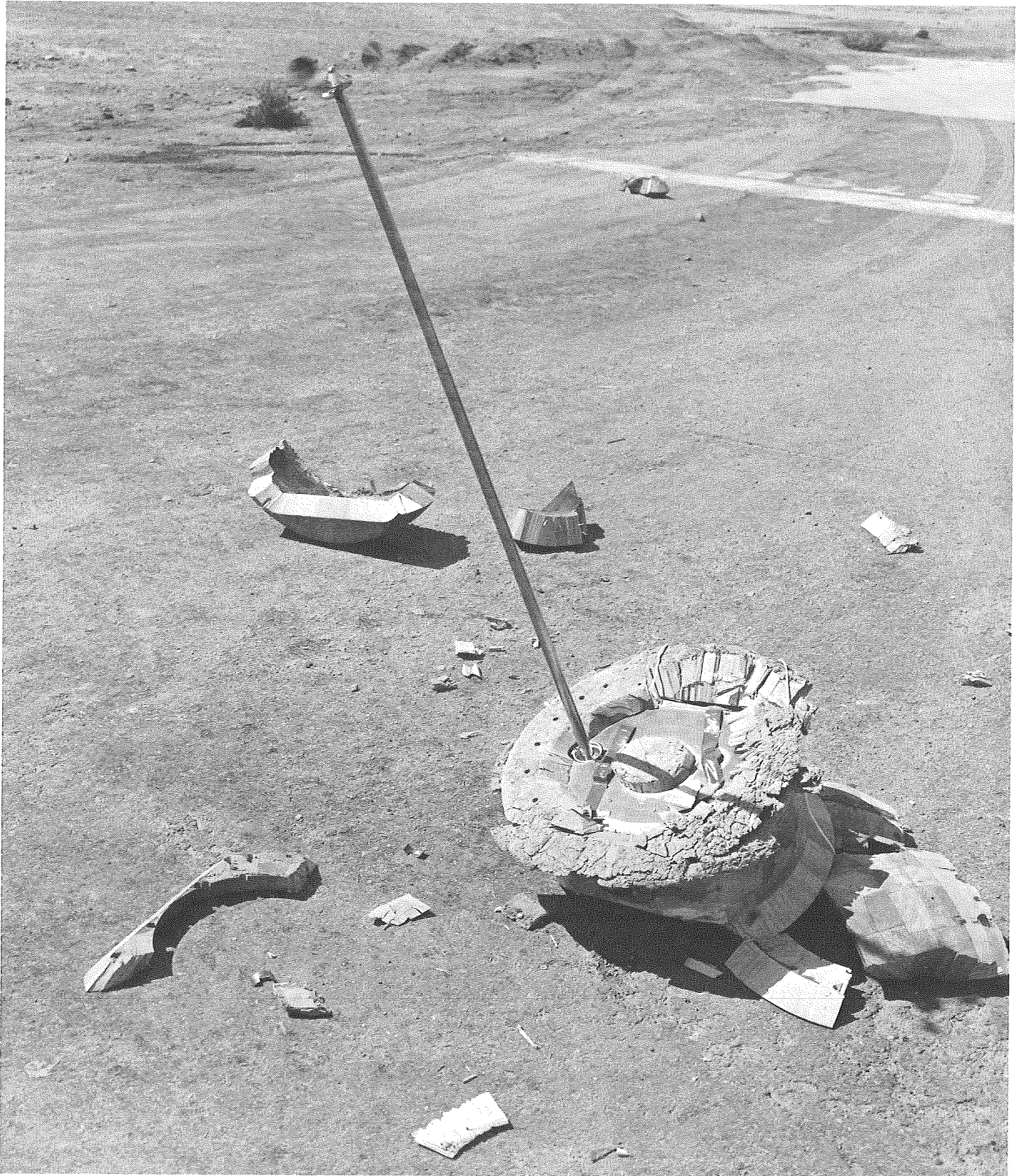
Fig. 5. Lander after drop on asphalt (nonyielding surface)
