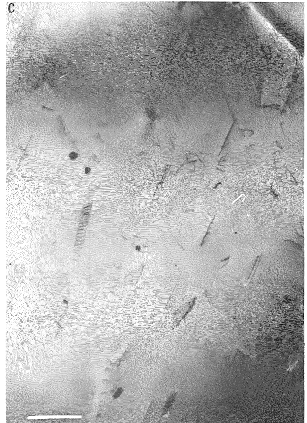
Figure 5. (A) Optical micrograph showing the microstructure of as-extruded Alloy 1 bar. 500x. (B) and (C) Thin foil micrographs of a cross section of as-extruded bar. Note the fine distribution of primary carbide particles and the low dislocation density. The line marks on the micrographs represent one micron.
