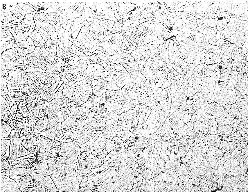
Figure 7. Optical micrographs of as-extruded and cold swaged Alloy 1 bar. (A) The cross section of rod as-extruded and directly cold swaged to .590 inch diameter. (B) Cross section of rod annealed for 8 minutes at 2200° F in the condition shown in (A) above and then further cold swaged to .460 inch diameter. Both at 500x.
