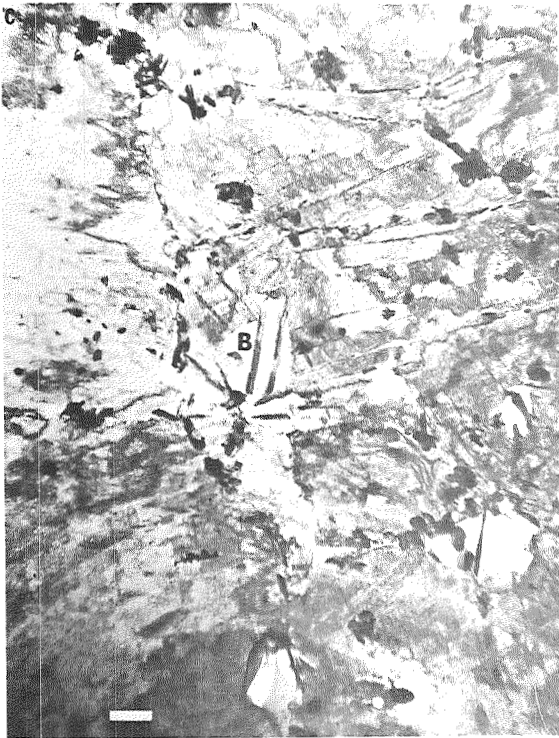
Figure 9. (A) Optical micrograph of Alloy 1 bar cold swaged to .460 inch diameter aged 120 hours at 1200° F and further exposed for 100 hours at 1400° F. 500x. (B) Plastic replica of Alloy 1 material as in (A) above. The regions marked "B" in Figures 9 (B), 9 (C) and 9 (D) seem to represent the beginning of secondary recrystallization. (See text.) Line marks on Figures 9 (B), 9 (C) and 9 (D) represent one micron.
