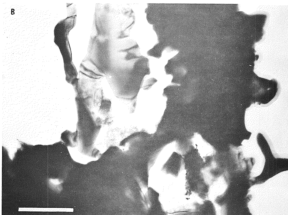
Figure 20. Thin foil micrographs of individual particles of alloy 2 powders (these transmission micrographs have been prepared by "holding" the particles against an electrolytic nickel plate as shown in Figure 2). The line marks represent 1 micron.
