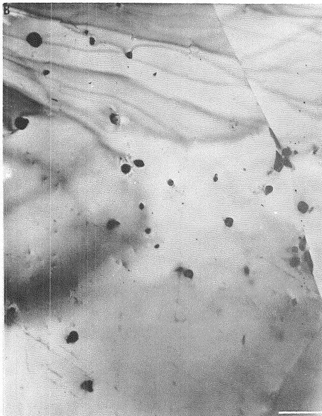
Figure 5. (A) Optical micrograph showing the microstructure of as-extruded Alloy 1 bar. 500x. (B) and (C) Thin foil micrographs of a cross section of as-extruded bar. Note the fine distribution of primary carbide particles and the low dislocation density. The line marks on the micrographs represent one micron.
