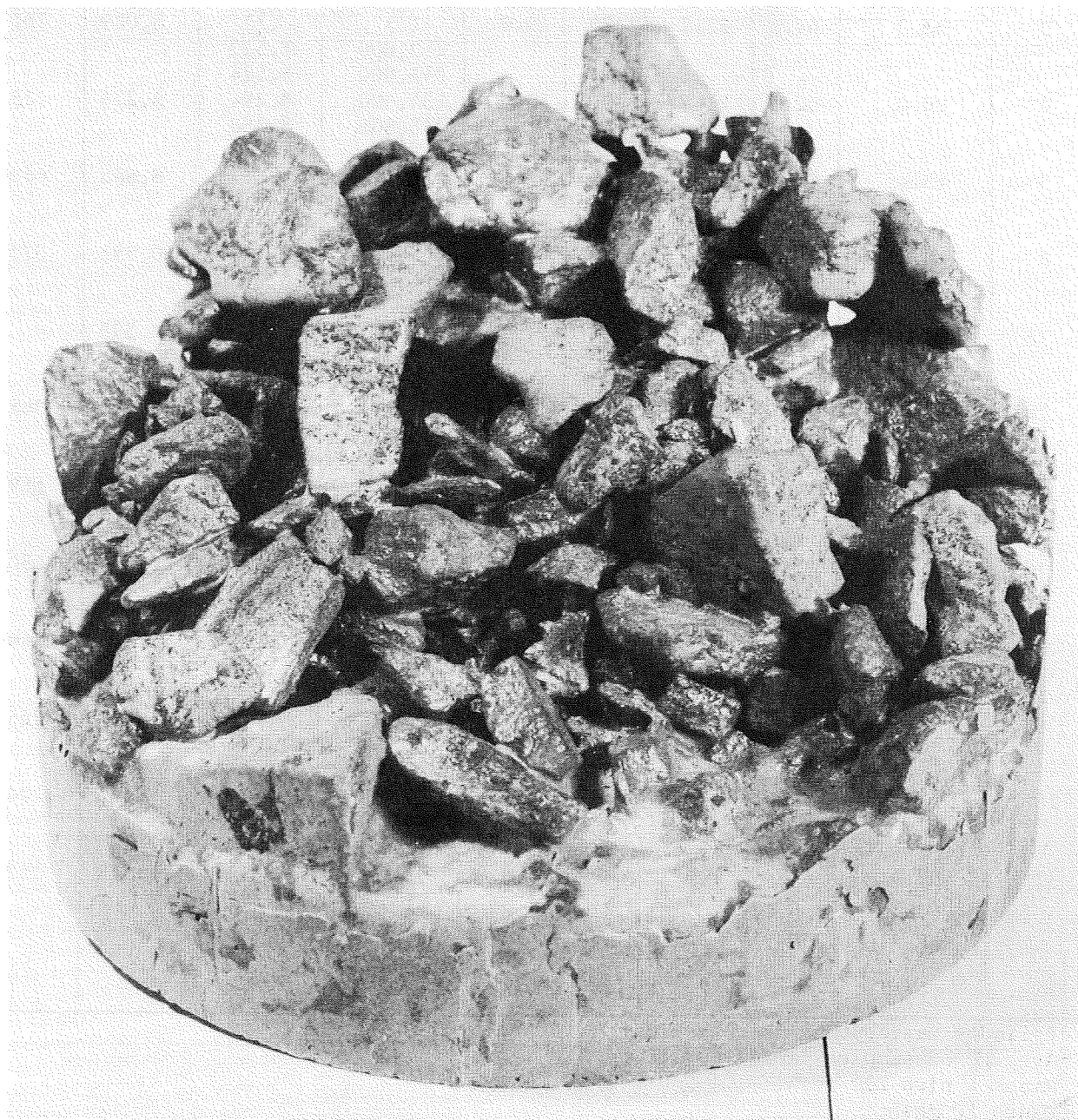
FIGURE 6. - Wetted and Partially Filled Coarse Aggregate.
