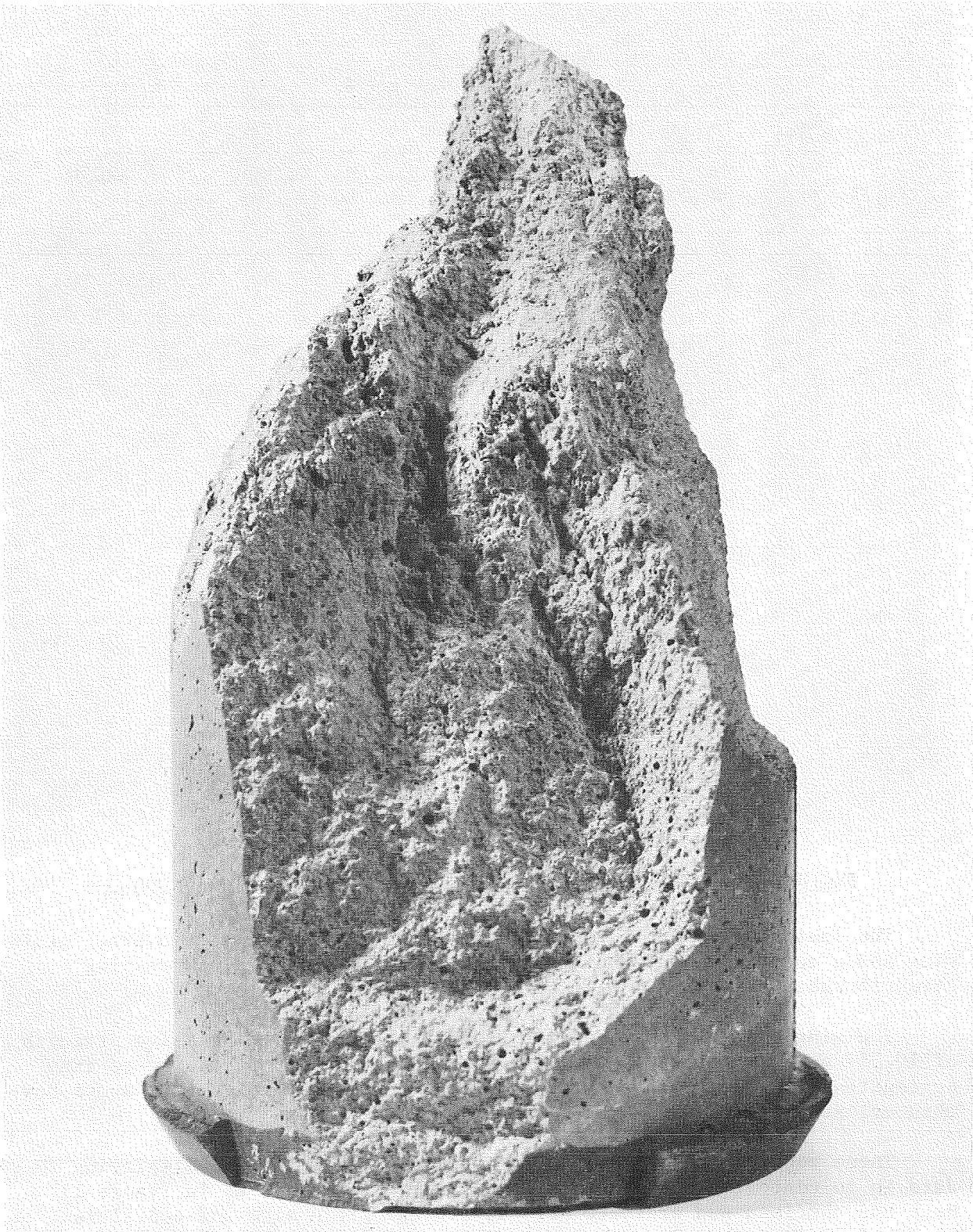
FIGURE 9. - Test Cylinder Using Excess Fines, Failed at 7,900 psi.
