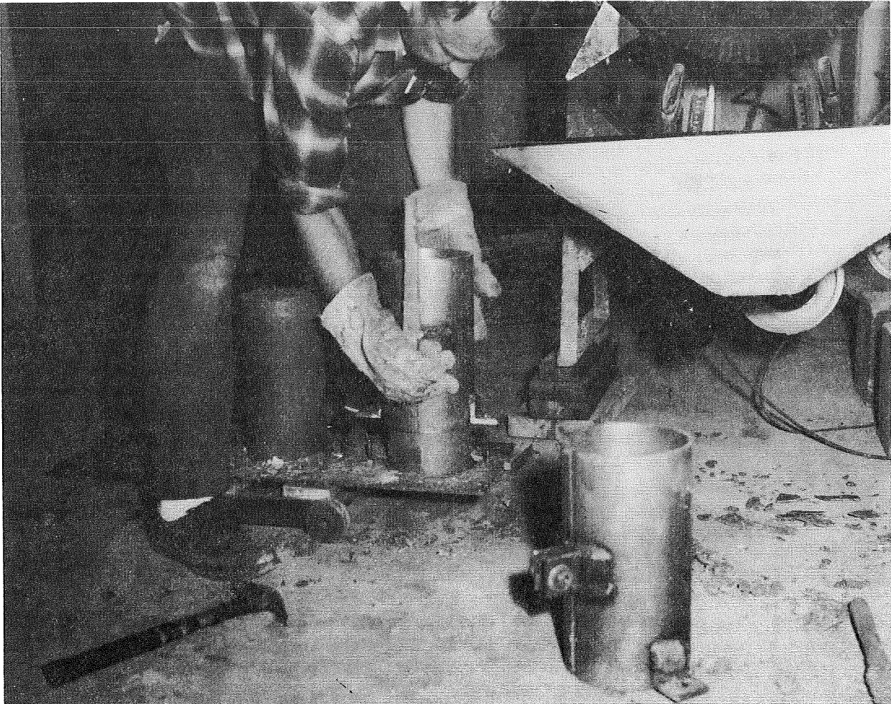
FIGURE 5. - Compression Test Cylinders (6- by 12-Inch) Being Removed From Mold.
