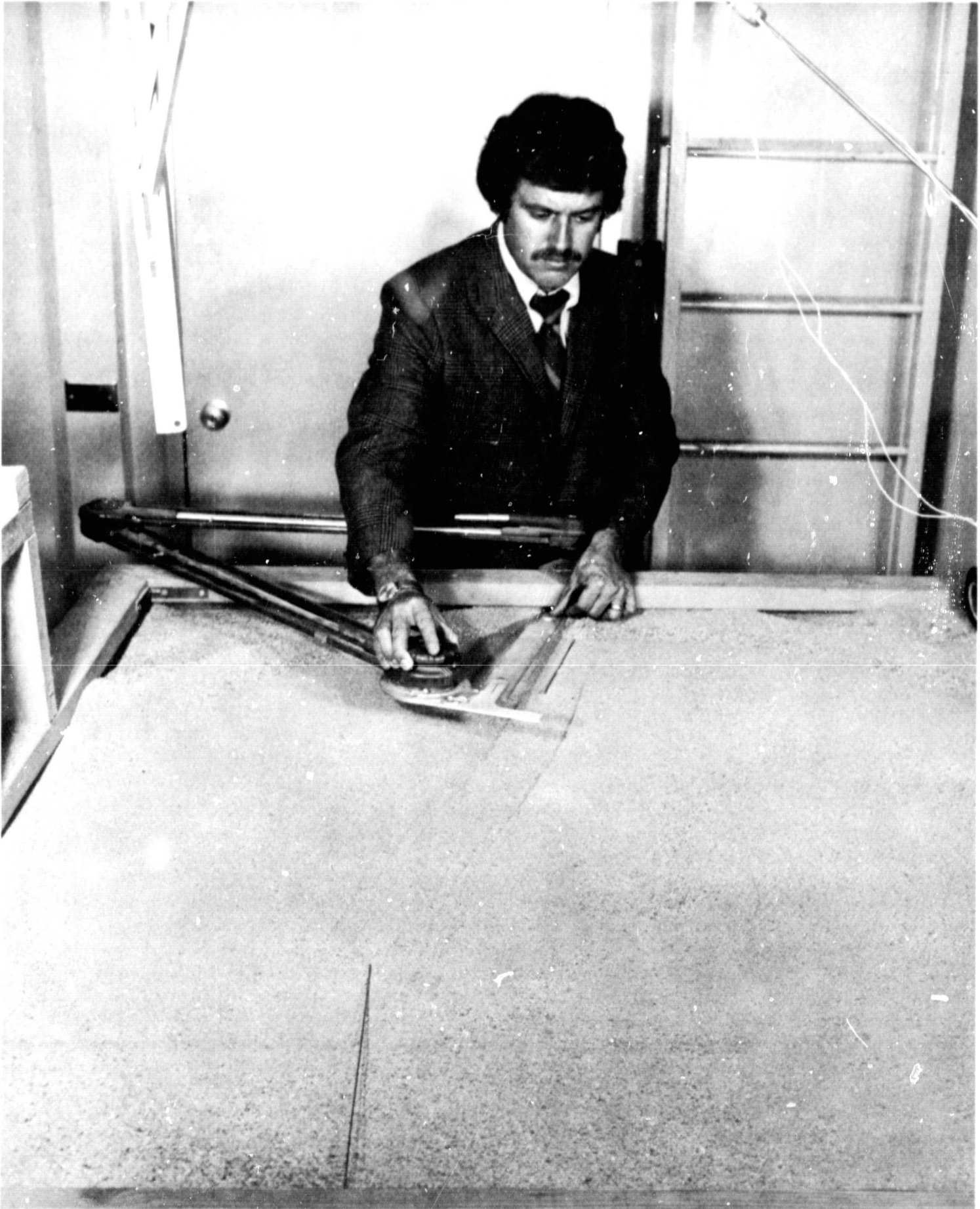
Figure 8. Procedure for Measuring Exit Angle of Vehicle
