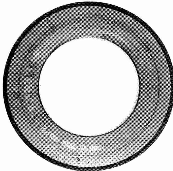
RETEST OF HYDRODYNAMIC FACE SEAL WITH OUTSIDE GAS-BEARING GEOMETRY AND CARBIDE ROTOR
