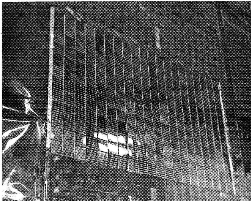
Figure 2.2-14. Spectrolab Module Mounted on G1 Blanket Assembly (VF 70-127D)
