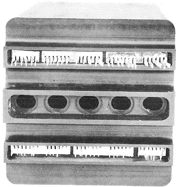
b) Copper Intercell and Intracell Connectors in Place (Photo A24855)
