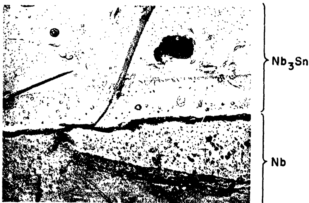
Fig. I-8. Etched cross-section of Nb-Nb 3 Sn interface showing a diffusion zone in Nb 3 Sn adjacent to niobium, which is indicative of Nb 3 Sn crystal growth by diffusion.
