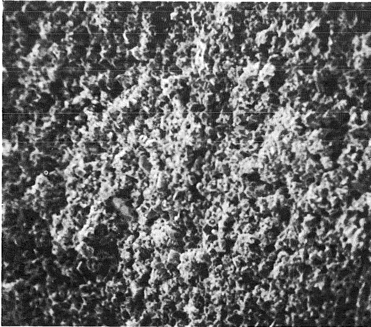
300 Magnification Silver Oxide Plate No. 35 As Received Flat Surface
