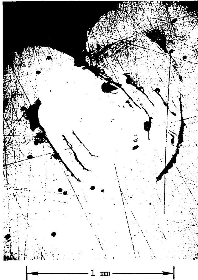
Figure 1.3. Damage Mark on a White Sapphire Plate Produced by Impact of a 2-mm Mercury Drop at 3.58 \times 10^4 cm/sec (1,175 ft/sec).
