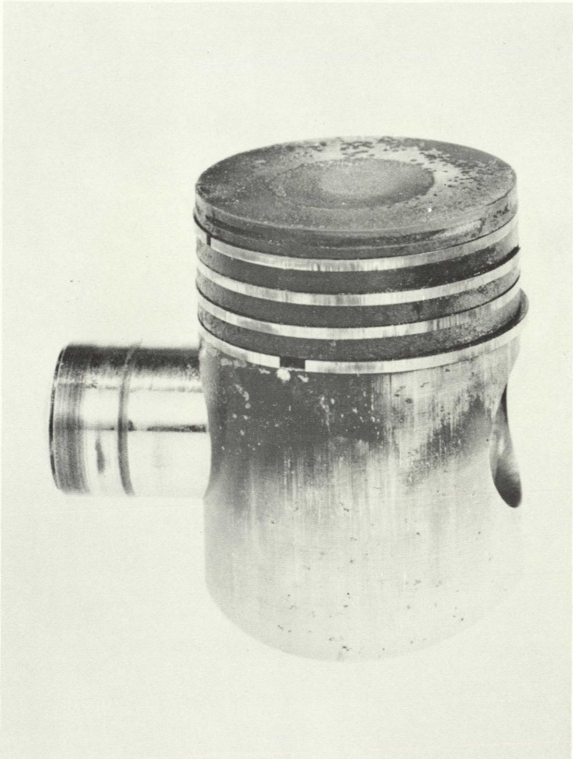
FIGURE 36. Modification 1 Piston Assembly after 90-hour Endurance Test
