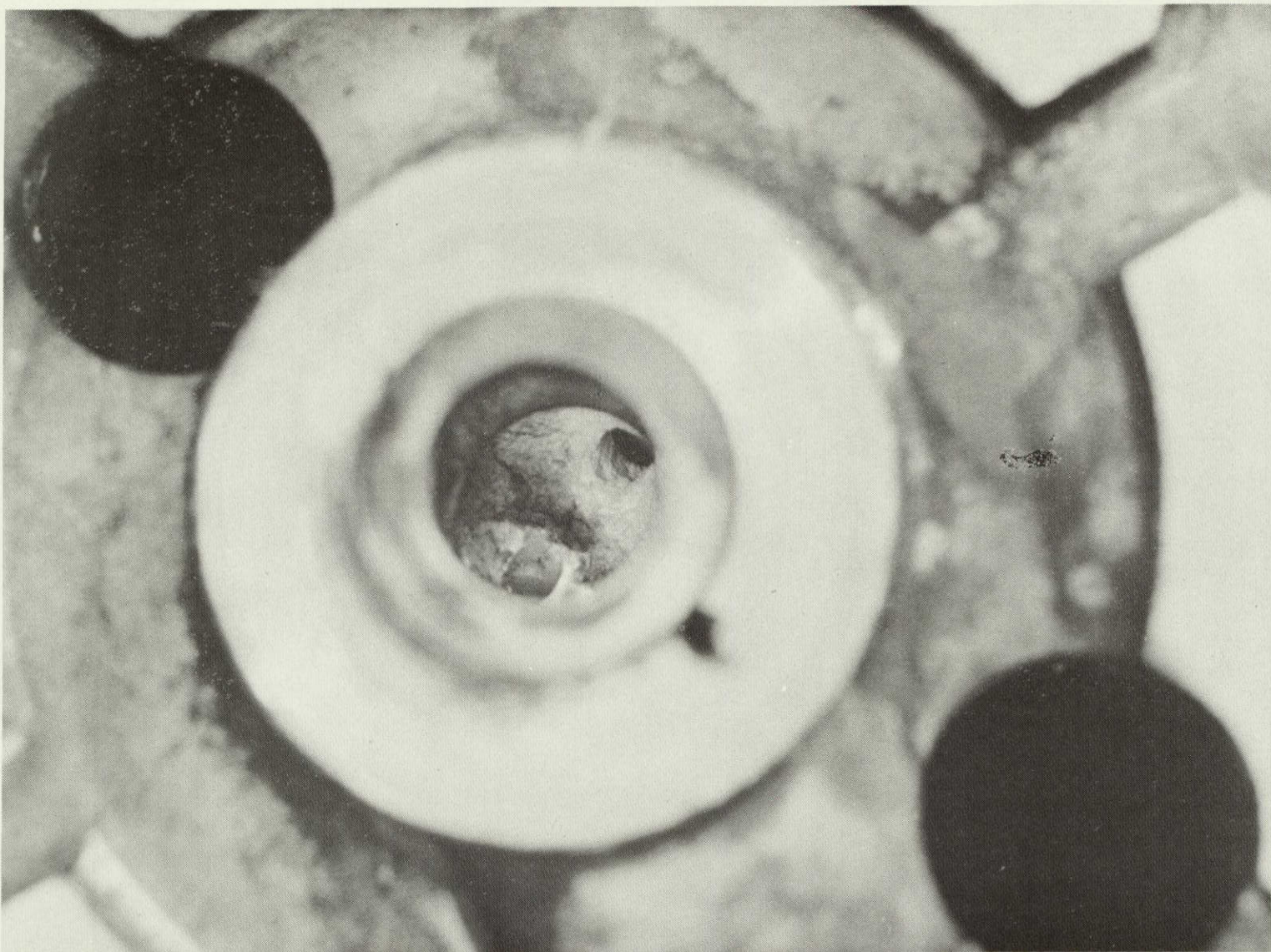
FIGURE 51. SPU-3 Cylinder Head Combustion Chamber after Test 5151-23
