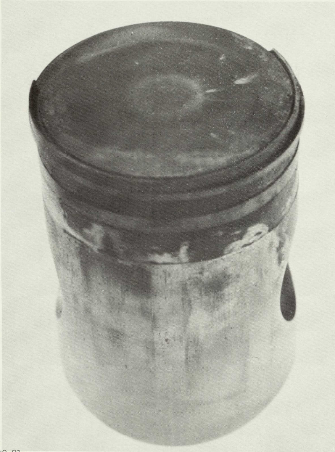
FIGURE 27. Configuration C Piston after Operation for 4.76 hours in the SPJ-2A-2 Engine
