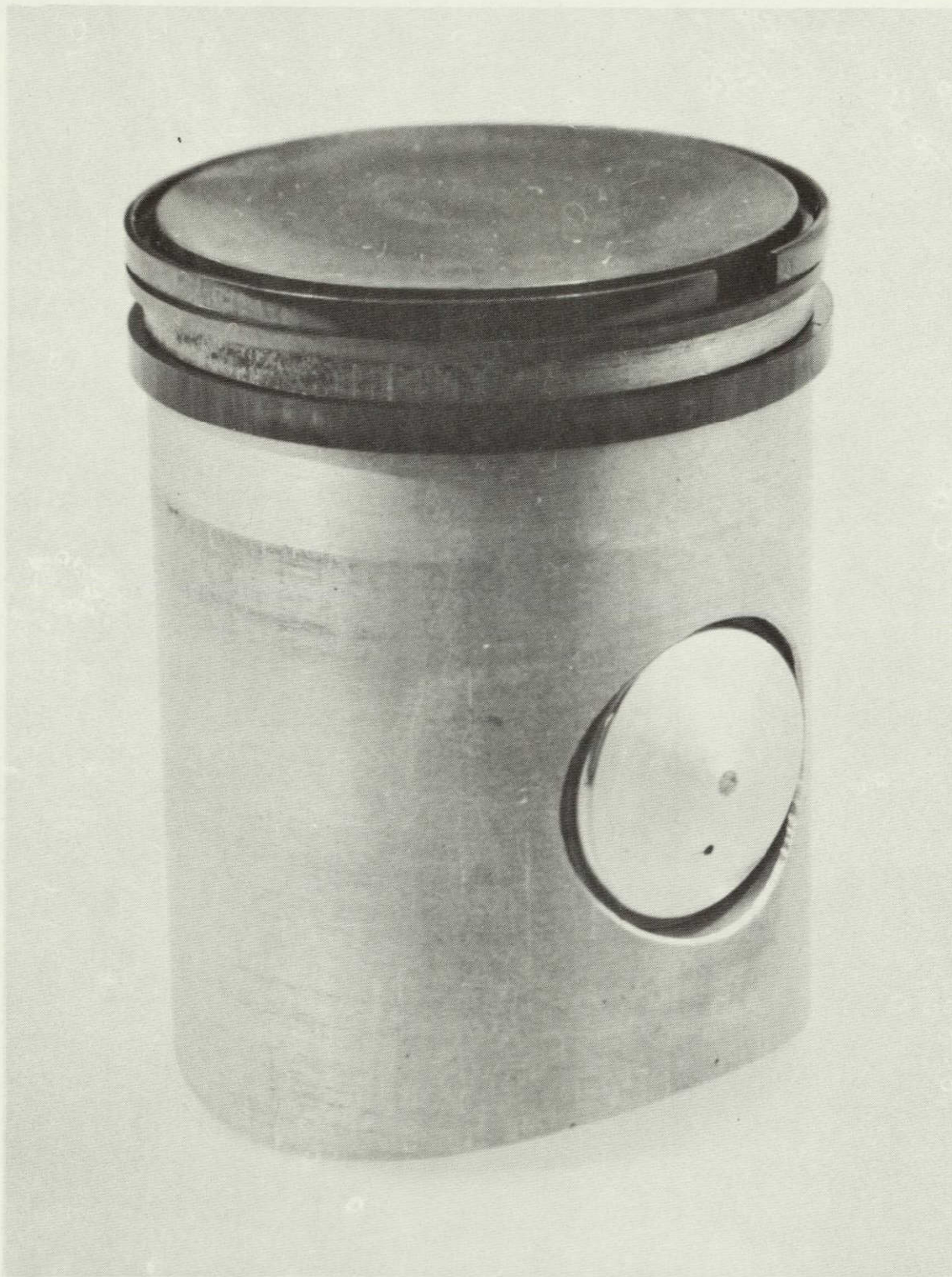
FIGURE 12. Baseline Piston Assembly Used in the SPU-3 Engine, After Test
