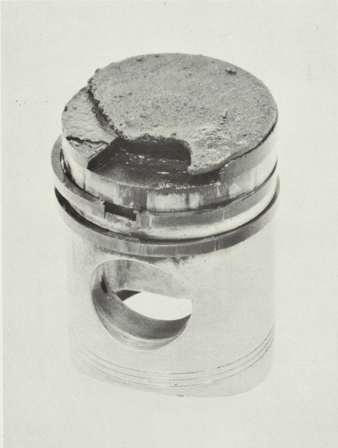
FIGURE 31. Insulated Crown Piston Configuration F after Operation for 0.3 hour
