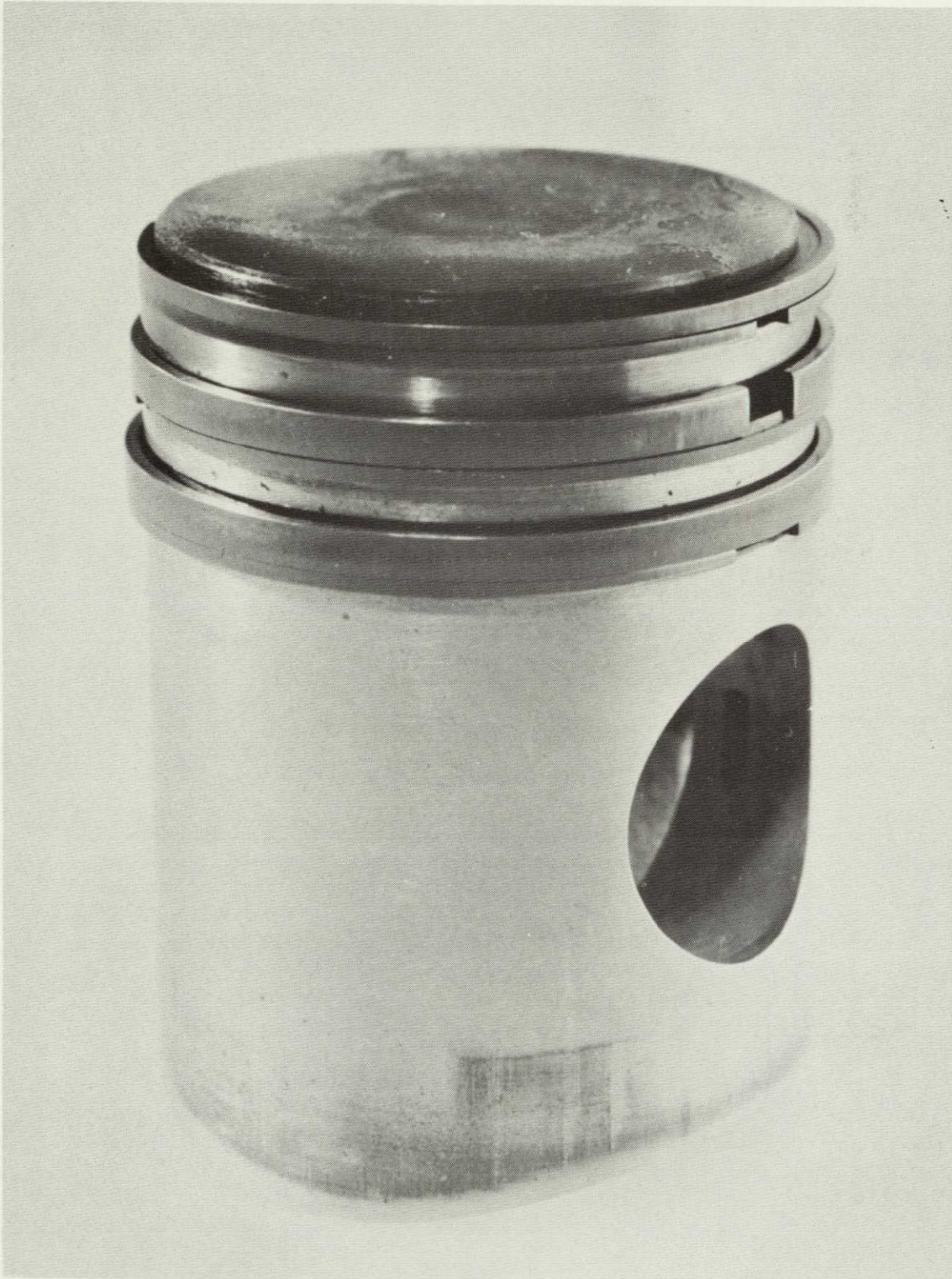
FIGURE 29. Configuration D Piston after Operation for 17 minutes in the SPU-2A-3 Engine
