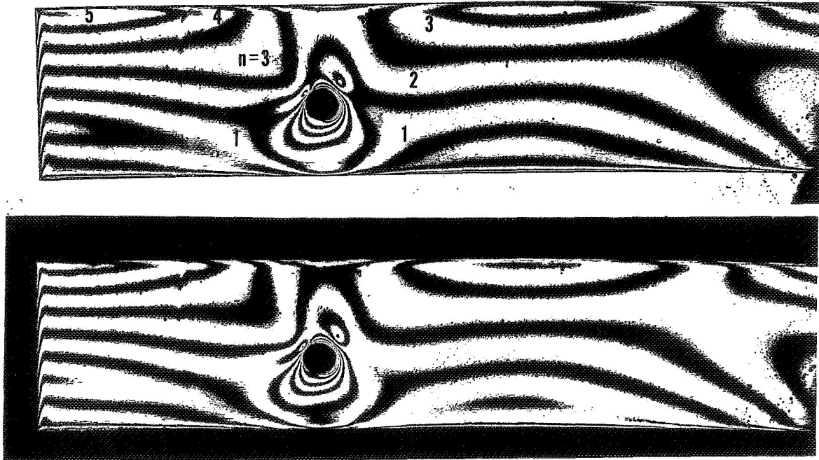
Figure 11. Frozen Stress Isochromatic Fringes, Model B (Light Field - Top, Dark Field - Bottom)
