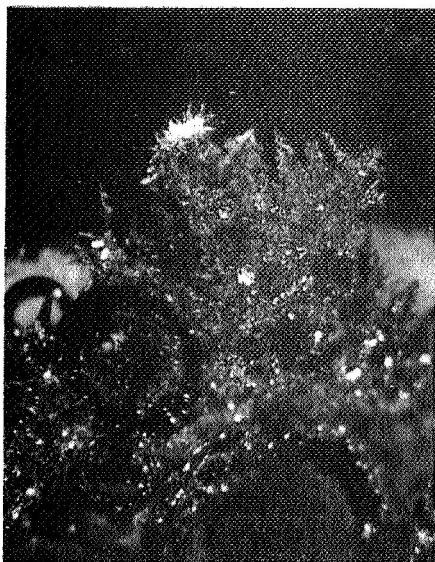
Fig. 39. Dendrites at Al electrode (25X) in \text{AlCl}_3 -KCl-NaCl (57.5-12.5-30 mol %) at 133 °C
