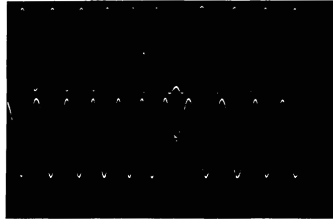
(b) Top: Signal Carrier (Point "c") with large figure error of approx. \lambda/4 Bottom: Reference Carrier (Point "d")
