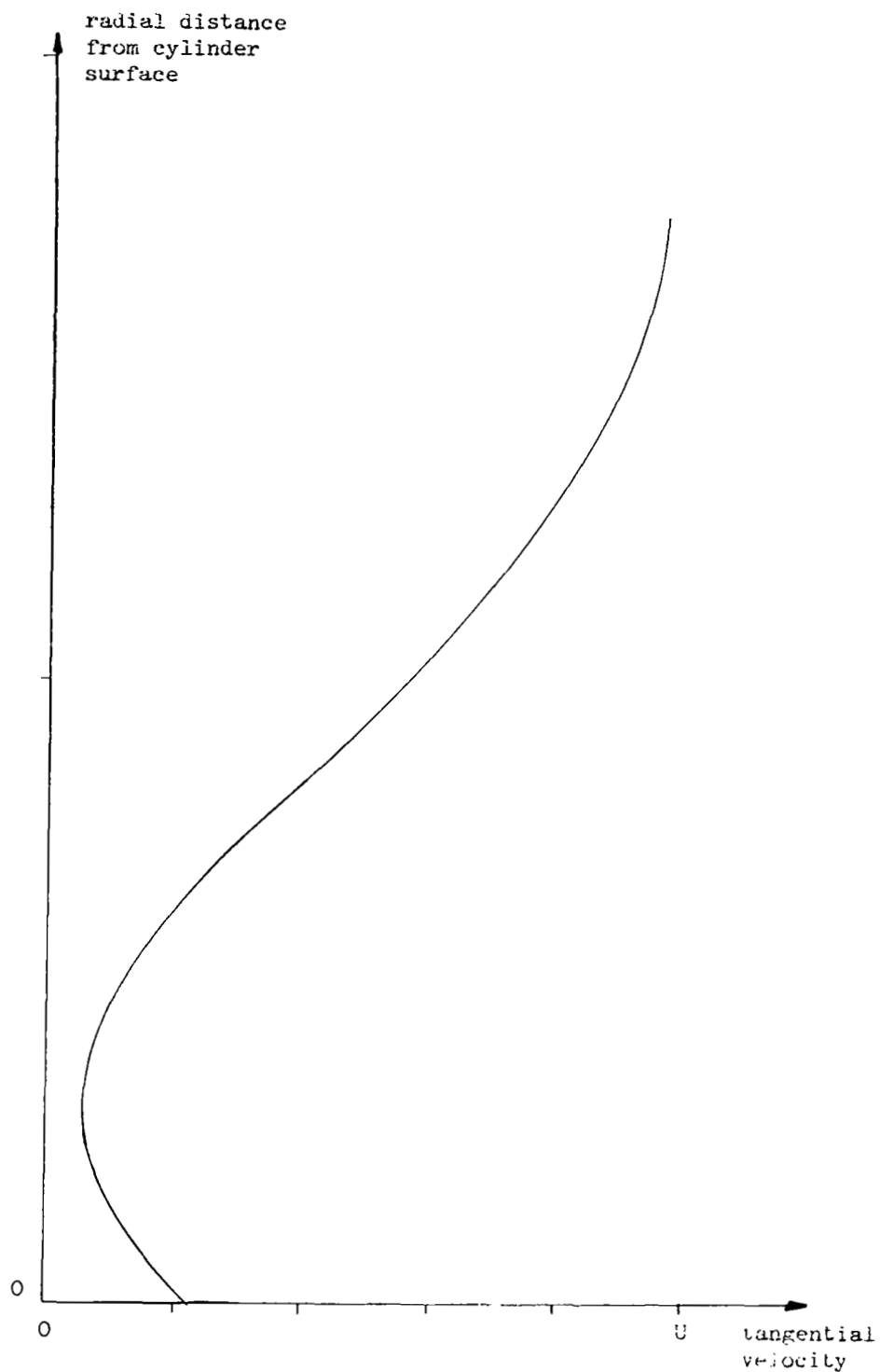
Figure 4. Profile near separation point above rotating cylinder from Brady and Ludwig.
