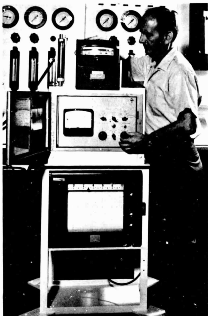
Figure 8.—Infrared apparatus for monitoring CO.
