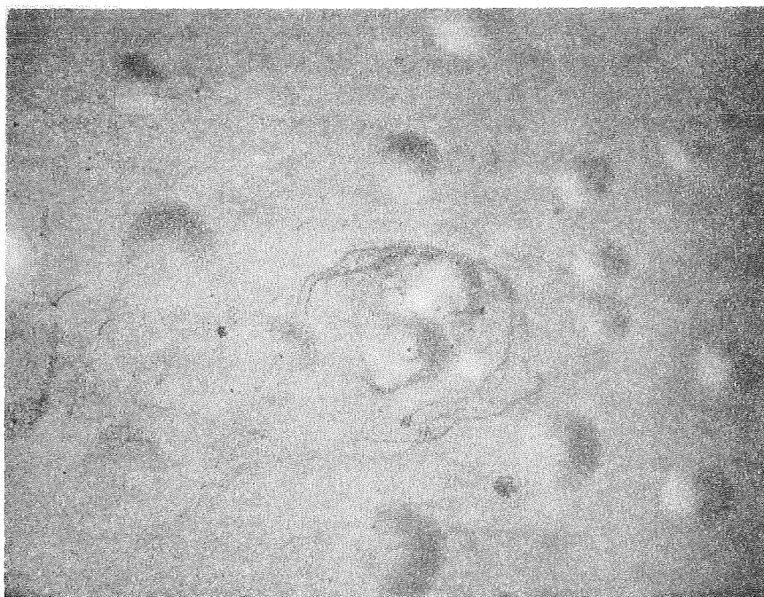
Figure 30: BLISTERS ON HELIOTEK SILVER-ON-SILICON SAMPLE (40X)
