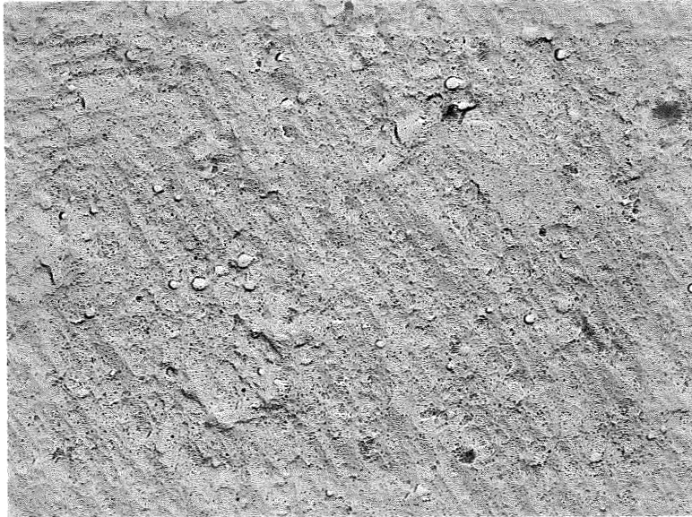
Figure 11. Electron micrograph of a replica of a TD Ni sample exposed 1000 hours at 1800 F (982 C) at ambient pressure. 30,000X
