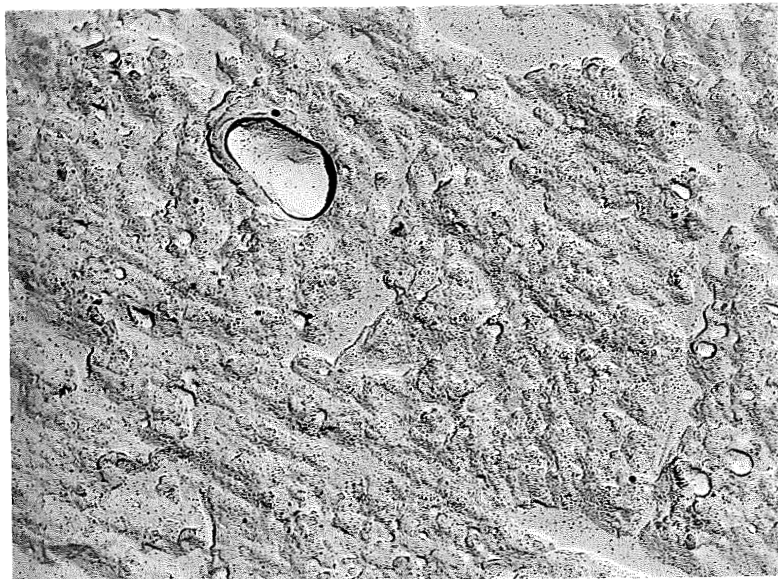
Figure 13. Electron micrograph of a replica of a TD NiCr sample after 3000 hours exposure at 2000 F (1093 C) and ambient pressure. 30,000X
