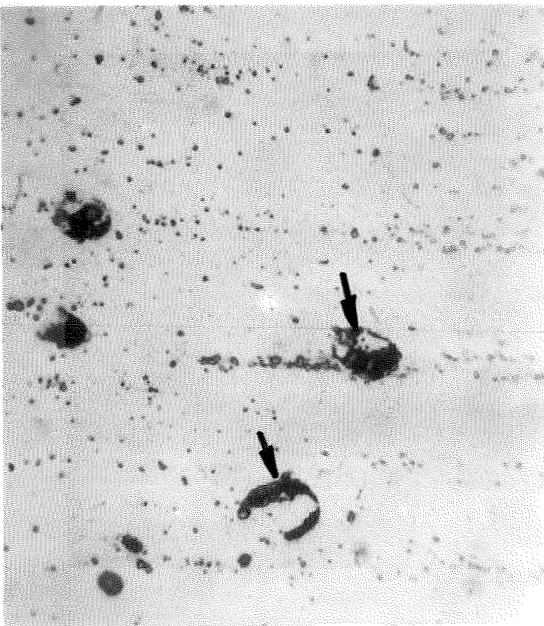
Figure 5. Oxide clusters in TD NiCr after 70 hours at 2000 F (1093 C) and 8 Torr. 800X
