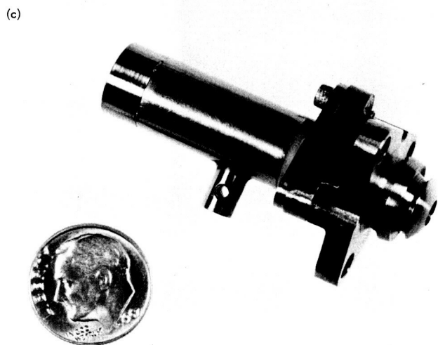
Fig. A-53. Avco ammonia thrusters: (a) assembly, (b) millipound prototype, (c) ATS-D/E micropound (photos courtesy of Avco)
