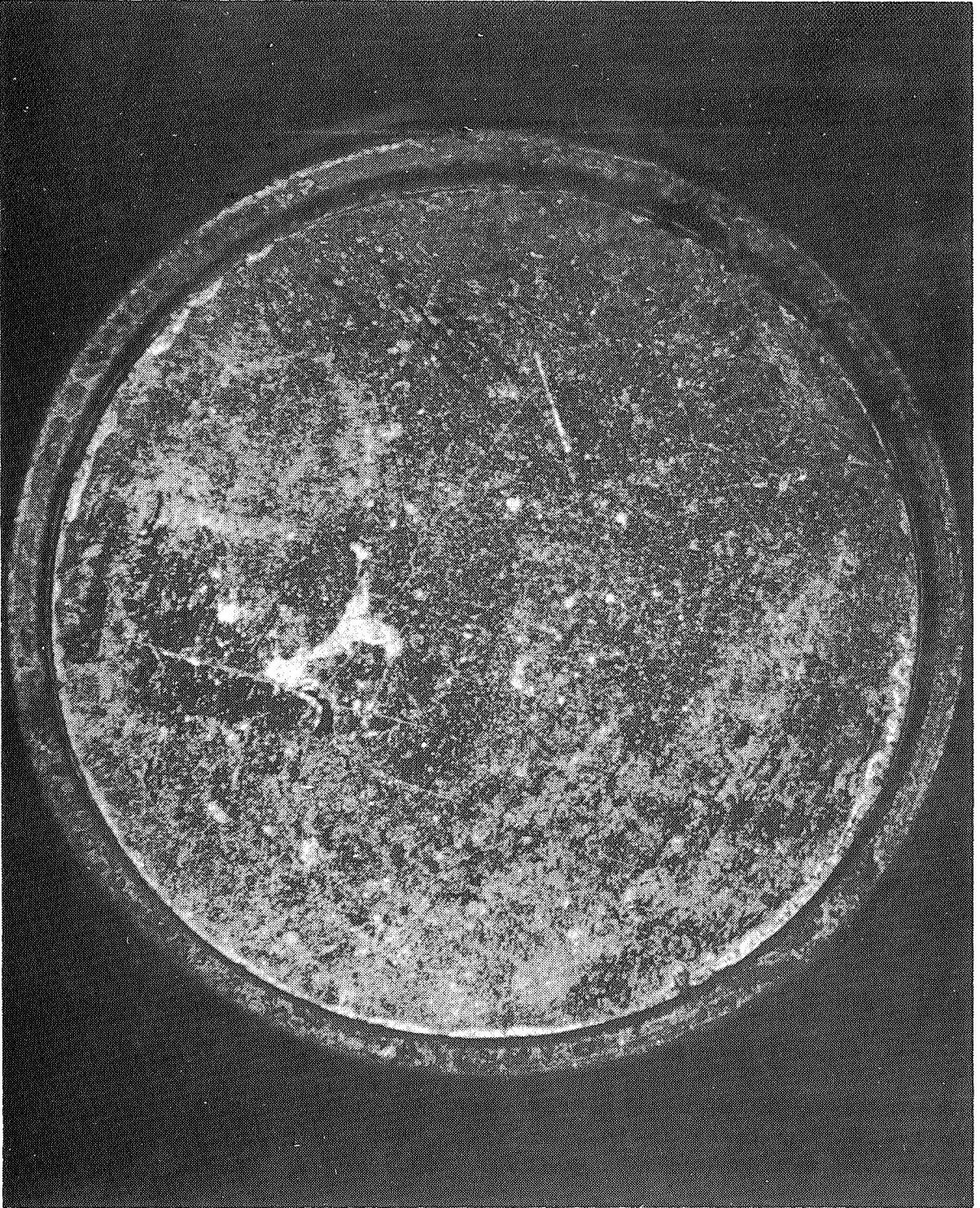
Figure 145. - Damaged diaphragm, pinhole failure.
