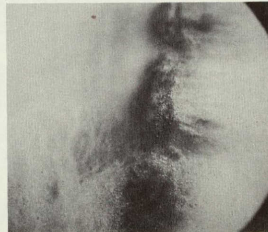
ELECTRODE SHAFT EROSION POST-TEST I-1 (15x)
