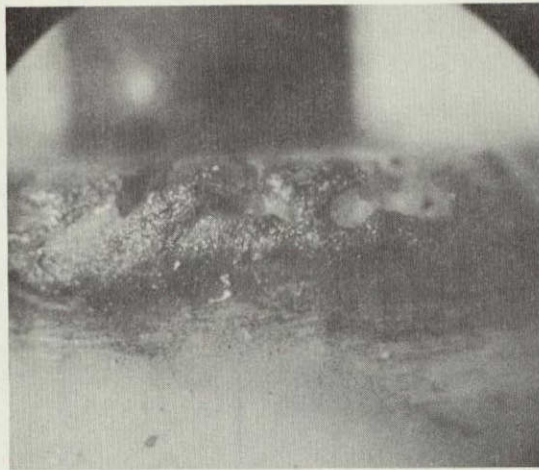
INSULATOR DETAIL - POST-TEST I-1 (15x)
