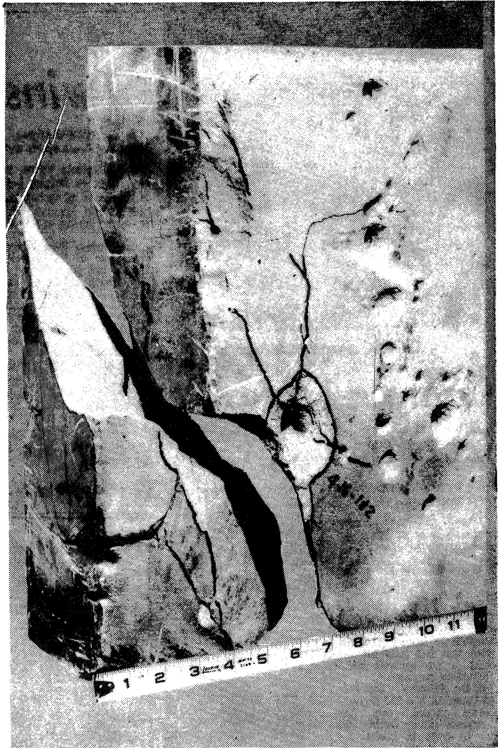
Sandstone fractured by jets of high pressure water
