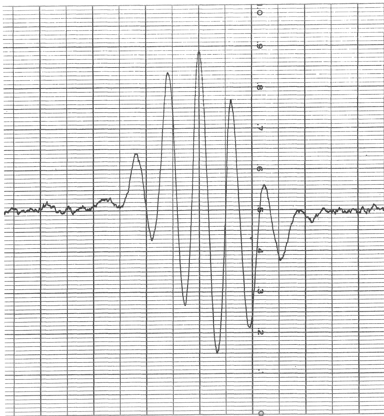
Fig. 104. Broadline ^{75}\text{As} Resonance in 1 M \text{LiAsF}_6 #1/MF #2-11 & 4 M DMF #7-3. One Division, Left to Right, is 1 Gauss.
