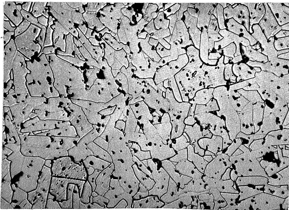
Figure 5. Etched Structure of SiC with 3 w/o Al 2 O 3 and 1 w/o C. Billet 1237, Density 3.08 gm/cc, Grain Size 8 μ.
