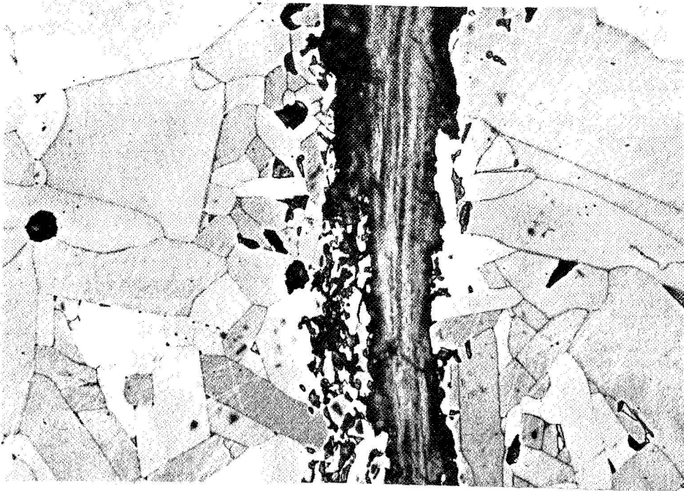
Figure 13a. Etched Microstructure of SiC Showing a Thornel Fiber in the Longitudinal Direction. Billet 1250
