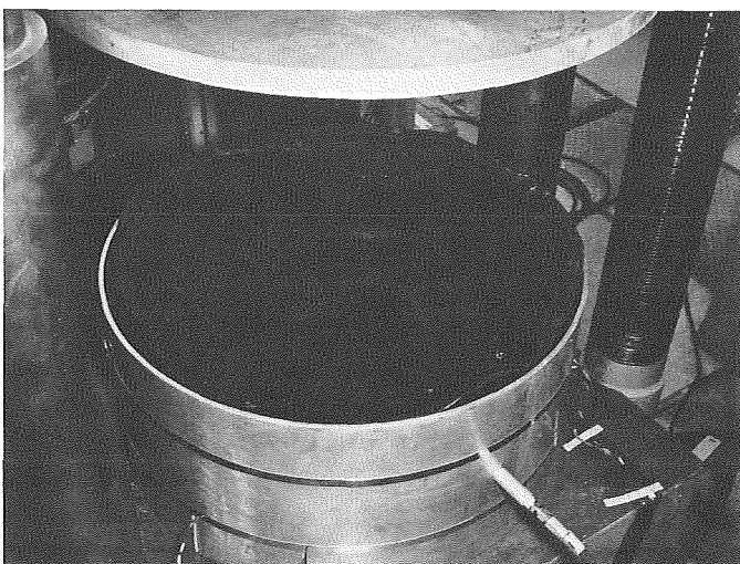
Fig. 22. Placement of pressure bag in compression fixture
