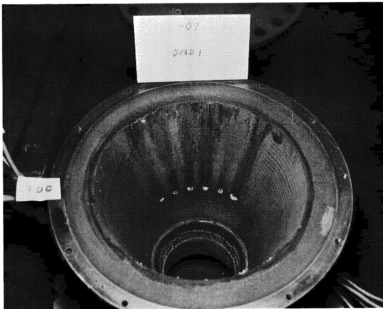
Figure 26. - Nozzle Condition, Quad I, Test 6107
