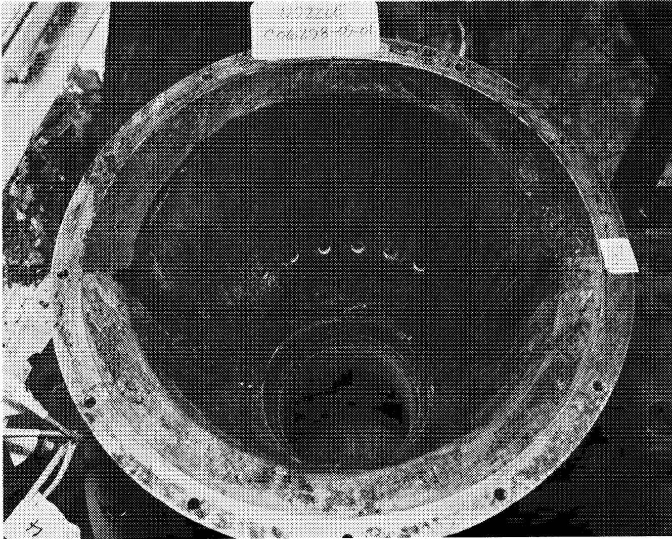
Figure 23. - Nozzle Condition, Quad III, Test 6105
