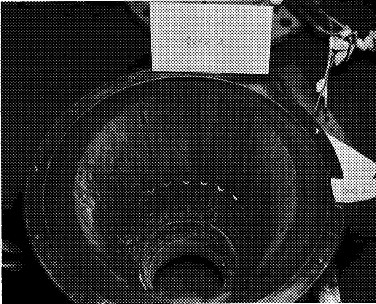
Figure 33. - Nozzle Condition, Quad III, Test 6110
