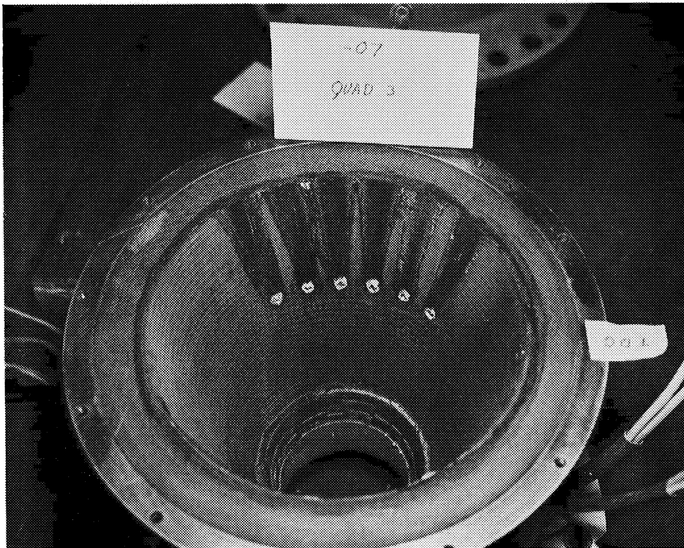
Figure 27. - Nozzle Condition, Quad III, Test 6107
