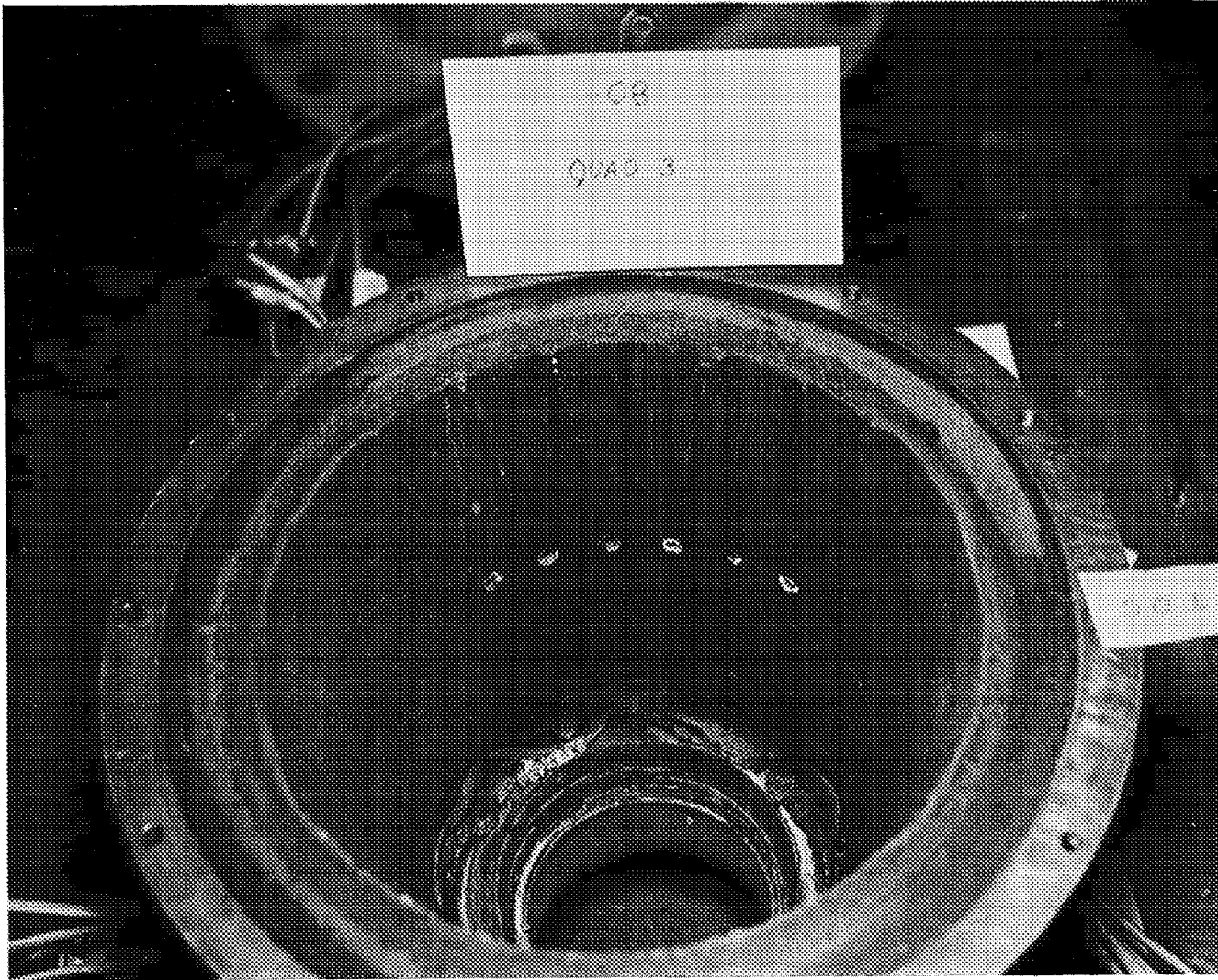
Figure 29. - Nozzle Condition, Quad III, Test 6108
