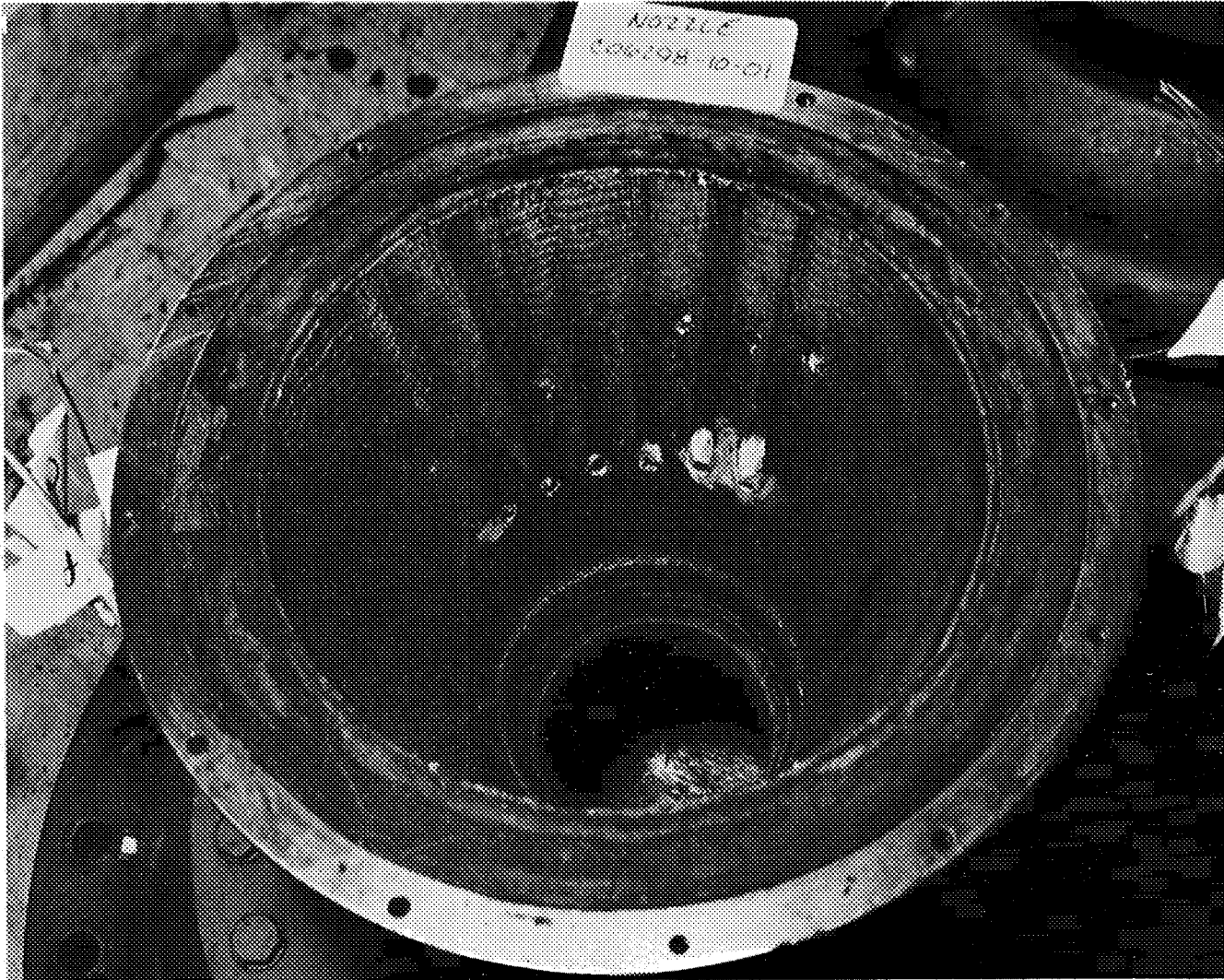
Figure 25. - Nozzle Condition, Quad III, Test 6106
