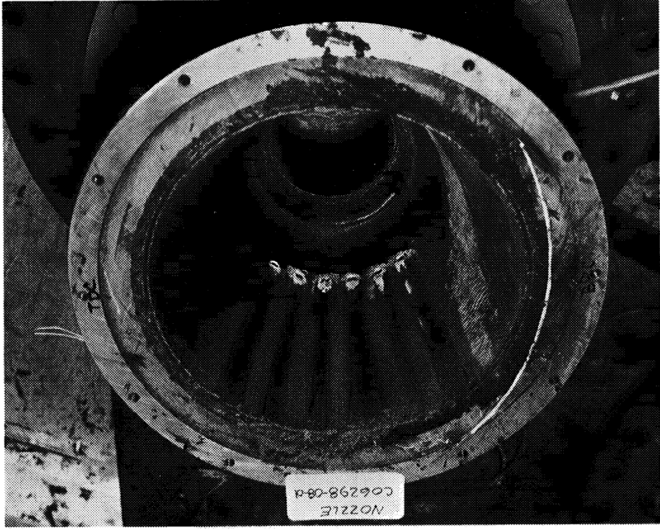
Figure 21. - Nozzle Condition, Quad III, Test 6104
