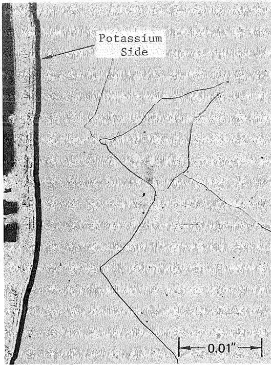
a. 3/8-inch OD potassium containment tube
