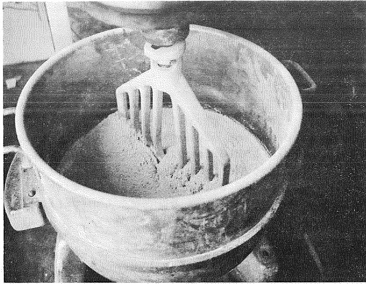
Figure 9. Mixing of High-Density Phenolic/Nylon Material
