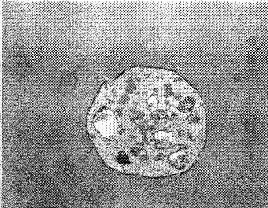
FIGURE 2. PYROLYZED R-1-50/FURFURYL ALCOHOL, 150 gram tension, plus 2 twists per inch, 200X.
