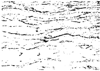
(f) As Rolled (76% Red.) 0.06" Sheet (385 DPH)
