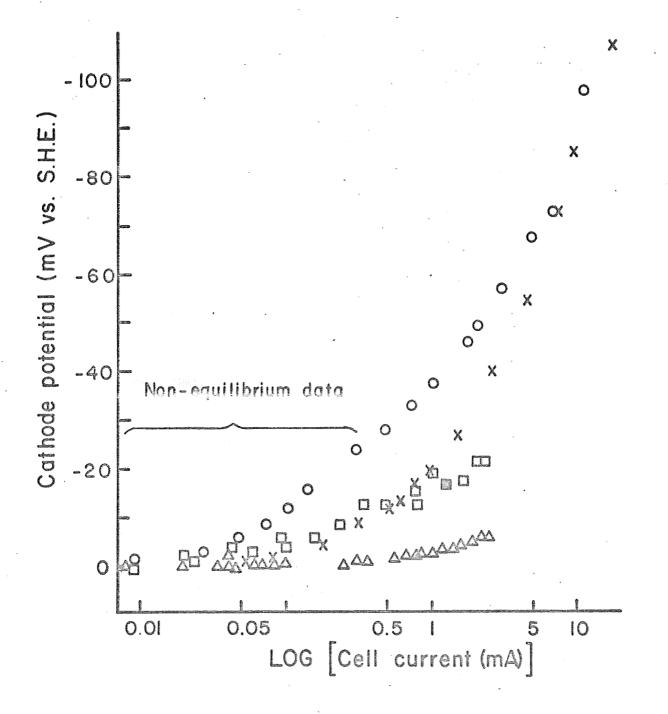
Effect of temperature on potential of the new three electrode reference system
