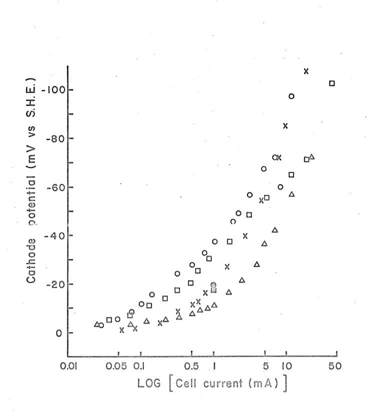
Effect of diffusing oxygen on potential of Giner type reference cathode at room temperature
