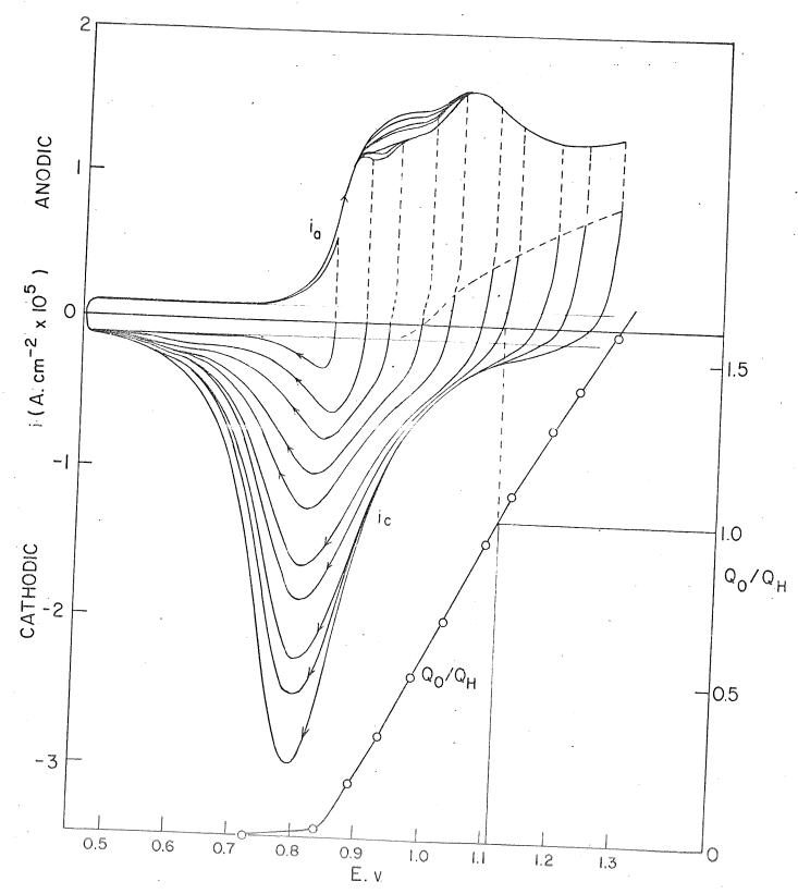
Dependence of cathodic peak potential  $\rm E_{p,c}~$  on extent of surface oxidation  $\rm Q_O/Q_H~$  and on corresponding potential .
