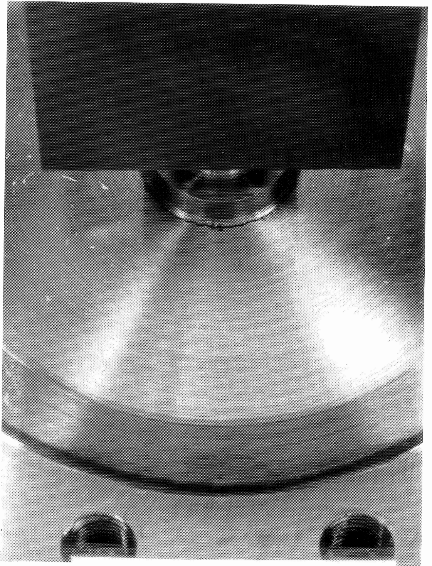
Diaphragm Failure Point As A Result of Destructive Burst Test
