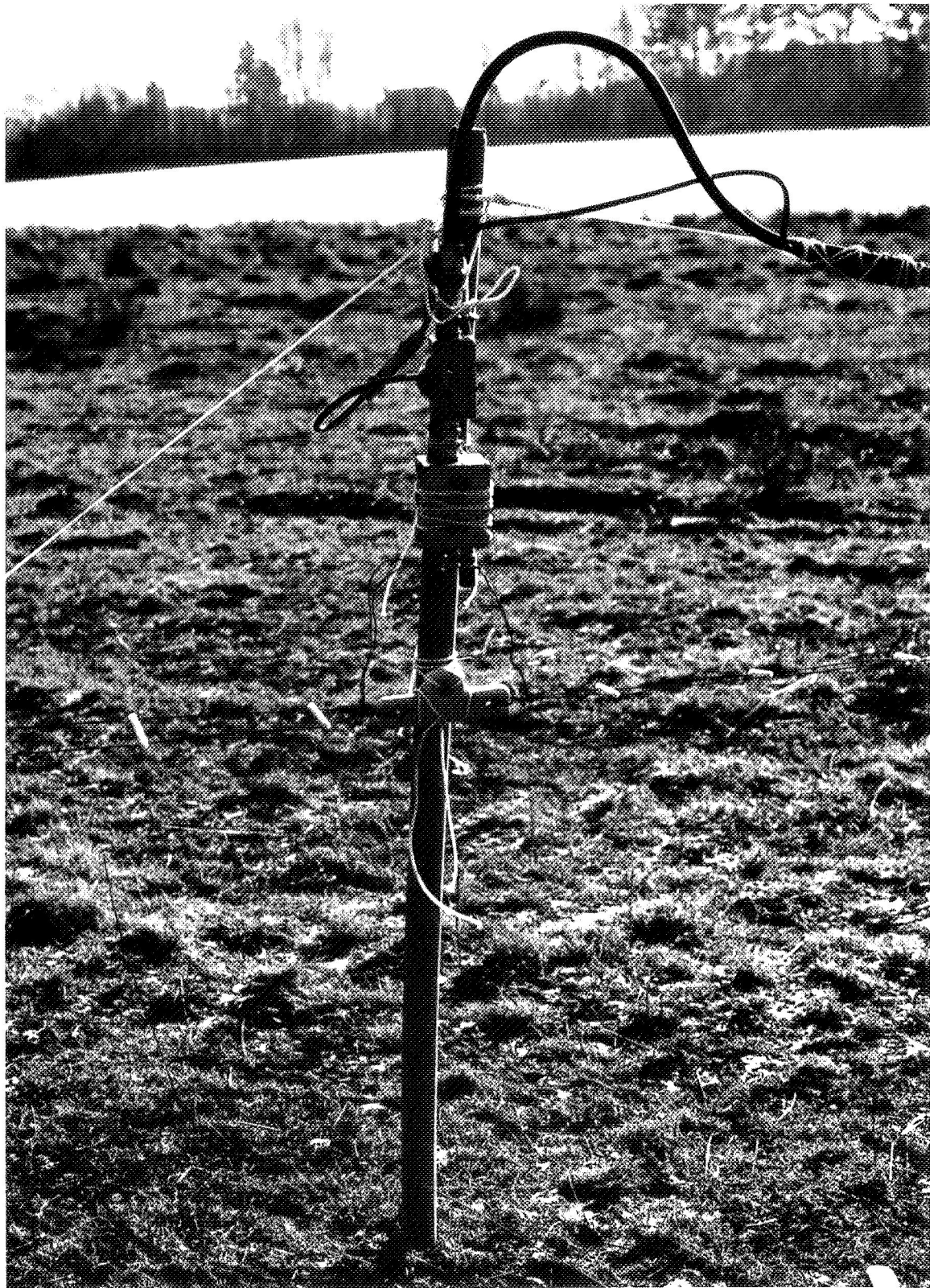
Fig. 11. Detail of North Receiving Antenna Construction. Two 15-meter lengths of 3-cm open-wire transmission line form the dipole antenna, connected directly to 200:50 \Omega balun transformer, thence directly to broadband RF preamplifier (gain 9db). RF transmission line (heavy cable) of RG9/U 50 \Omega coax is 204.8 meters in length for each of 4 receiving antennas, regardless of position. DC power for amplifier (20 V, 40 mA) is supplied over variable length of RG 58/U cable.
