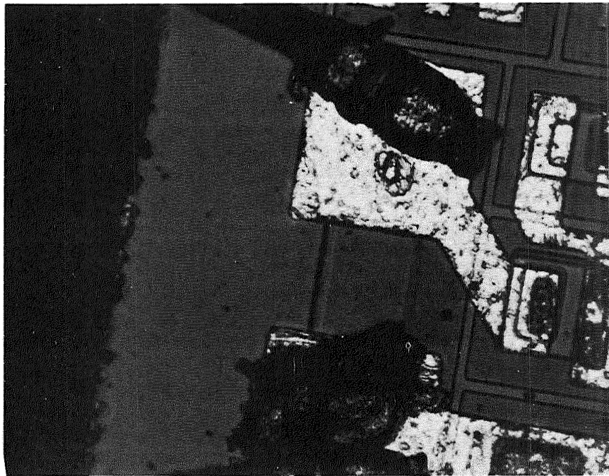
Figure I-16. Surface Photo of Type MIC 936 Failure Device Showing Dual Bond on Pad
