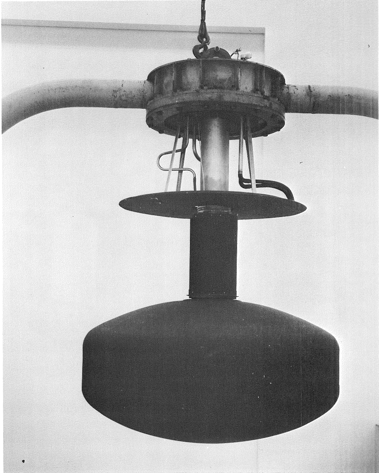
Fig. 3-2 Tank Calorimeter Supported in Handling Fixture
