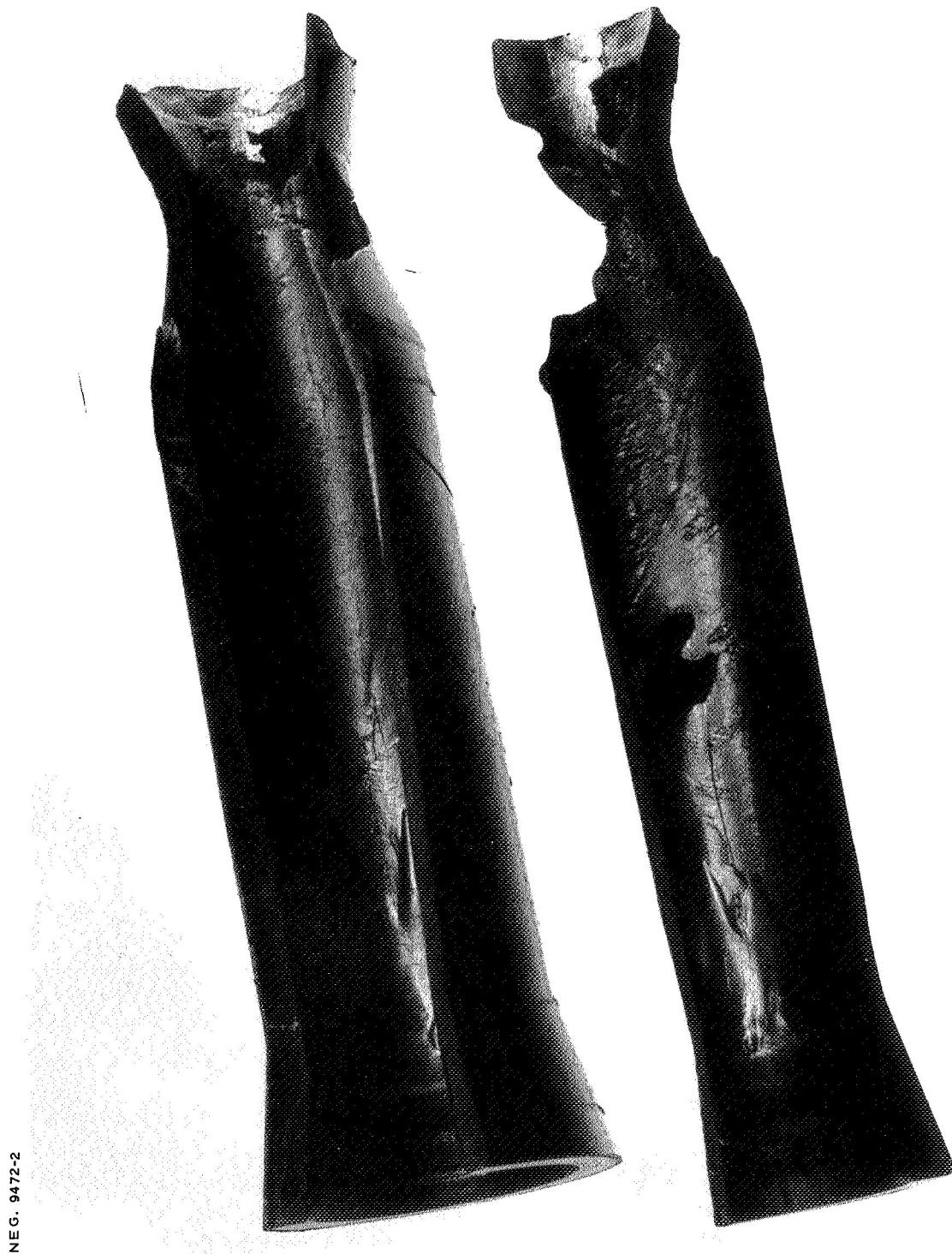
FIGURE 56. PG/Carbitex Chamber with RPG Nozzle Extension after 322 Seconds Firing
