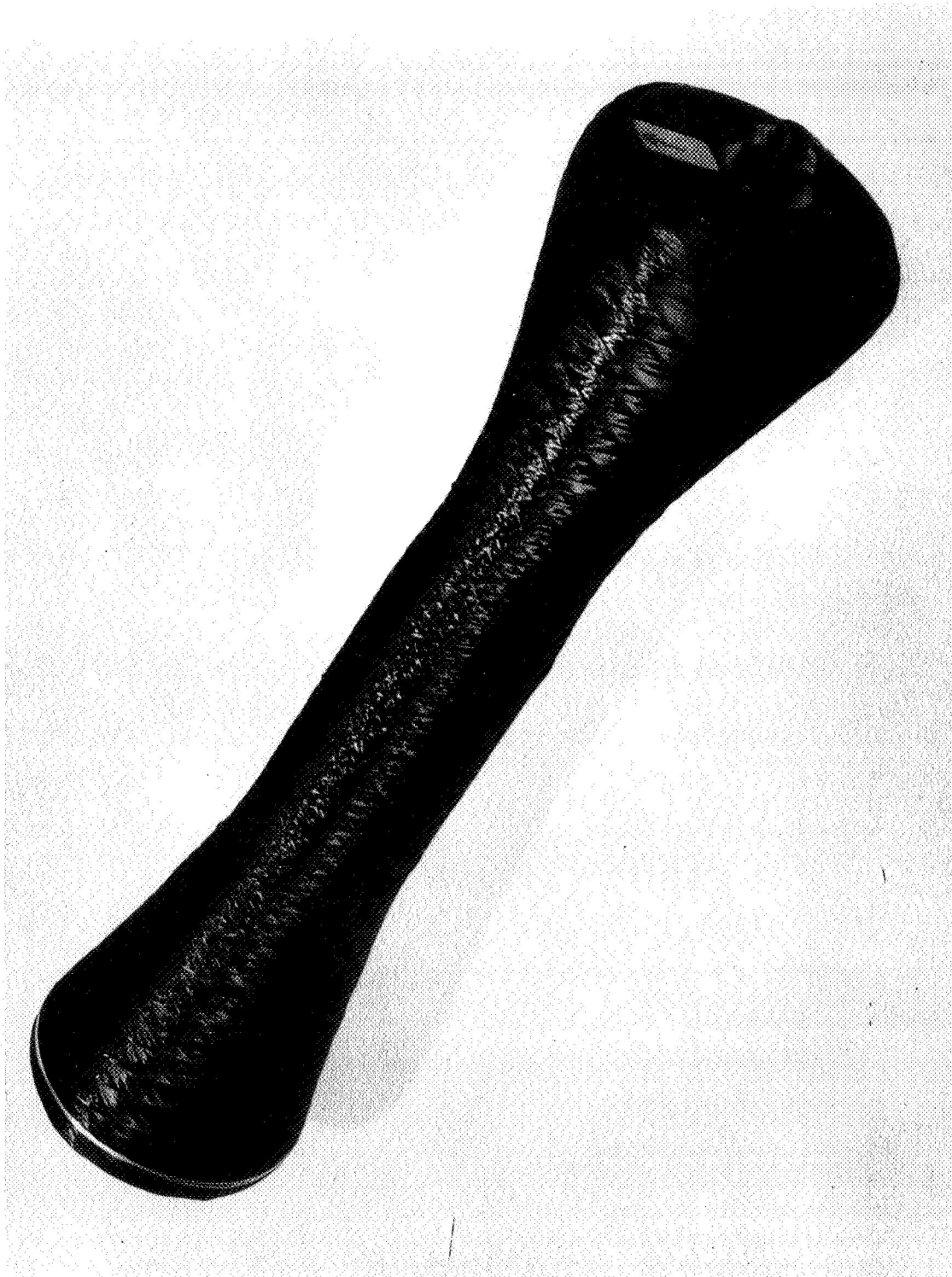
FIGURE 40. Thornel Wound Altitude Chamber before PG Infiltration
