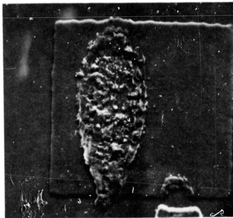
b. Lift-off at weakened weld. Magnification: 500 x.
