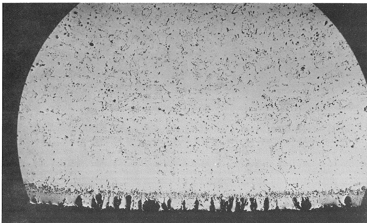
Figure 18. Ballistic Impact Sites 1900°F (1310°K) Impact on Al + Y Metallide System After 200 Hours Static Oxidation at 2000°F (1367°K) (F 6009, F 6010, 50X).
