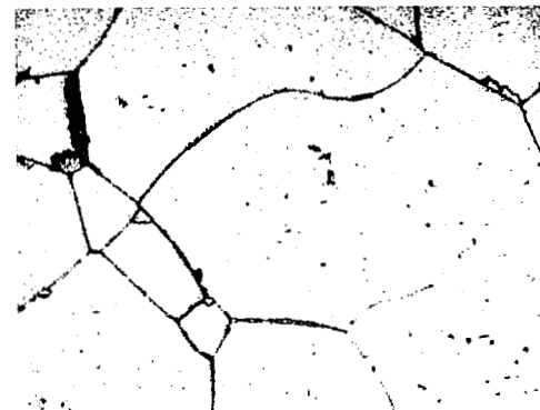
(g) Base Metal (Point H in Fig. 70) 500X 345 DPH
