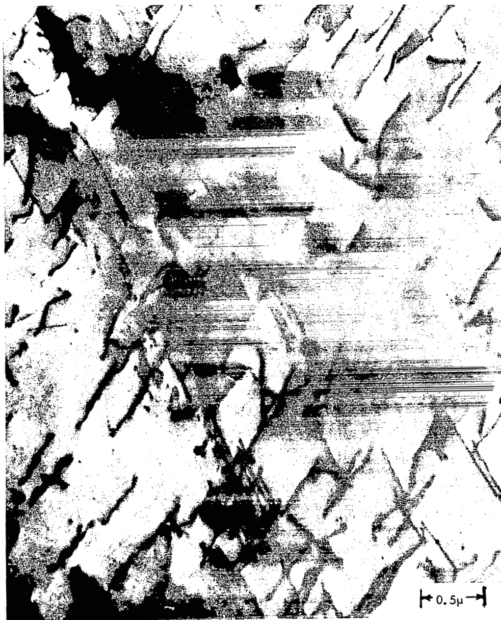
FIGURE 55 - Electron Transmission Photomicrograph of ASTAR-811C, Annealed 1 Hour at 3630°F, Then Tested at 2400°F and 15,000 psi. Test Duration 1000 Hours. Total Plastic Strain 2.5%.
