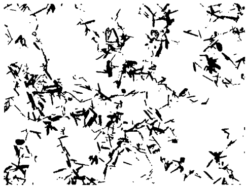
FIGURE 53 - Electron Micrographs of Tantalum Dimetal Carbide ( Ta_2C ) Precipitate Extracted from ASTAR-811C Specimens, Creep Tested at 2400°F and 15,000 psi
